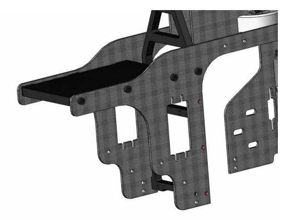
Now we will attach the radio tray. There are 3 M3x8 cap head screws needed for each side.
