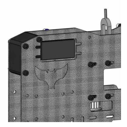
Attach the rear cross member to the helicopter using six M3x8 cap head screws.
