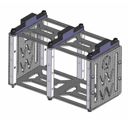
Assemble the fuel tank assembly as shown. Use M3x12 cap head screws on the top 6 screws. Slide the complete fuel tank into the cage and secure it in place with the lower plate. The front two plate holes are secured with M3x10 cap screws. The front and rear QWW plates are optional. You can leave these off to save weight if you want. The QWW plates are not included on the budget series bat helicopters.
