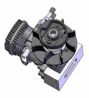
Next, attach the clutch shoe to the fan hub.
