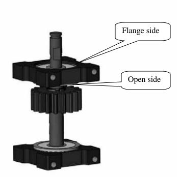
Next, install the two counter gear bearing blocks. Be sure that the flange face the top on the upper block and down on the lower block.
