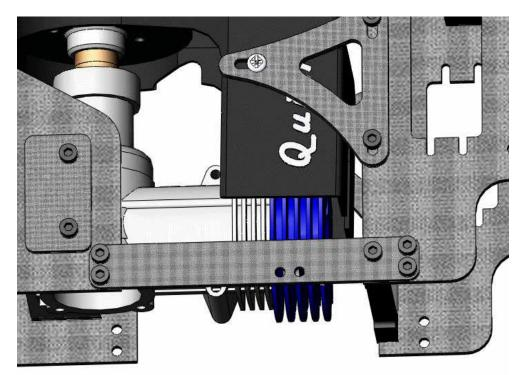
Four bolts will go through the plate and be attached with the lock nuts and the fifth will go into the bulkhead.
