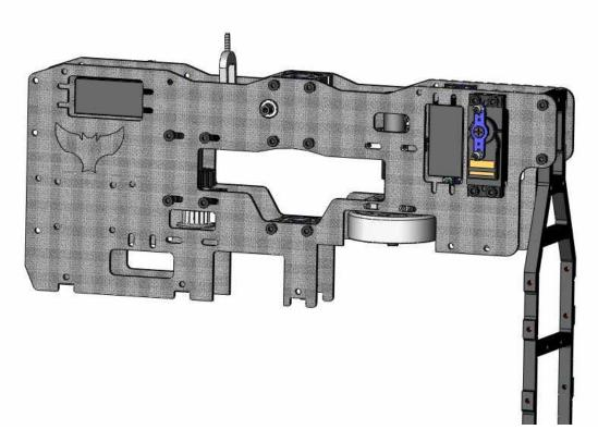
Now attach the two frame halves together. Use (4) M3x8 cap head screws to attach at the Counter gear assembly. Use (6) M3x8 cap head screws for attaching the main shaft bearing blocks. Locate your 2<sup>nd</sup> clutch bell bearing block doubler. Use (2) M3x10 socket head cap screws to attach the upper bearing block on the clutch bell assembly to the main frame. Use (2) M3x10 button head screws to attach the clutch bell assembly's lower bearing block.
