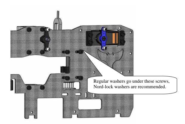
Now attach your counter gear assembly using (4) HHI3M08C (3 X 8mm SOCKET HEAD CAP SCREW) screws. Leave this slightly loose until you are ready to adjust gear mesh. Included are 4 M3 washers to use on the slots. It is recommended that you upgrade these to M3 Nord-lock washers to prevent any bearing block movement than can result in the main gear stripping out.
