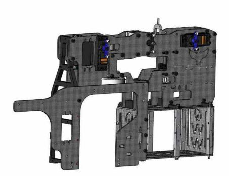
Next attach the lower engine frame. There are three M3x8 cap head screws in the rear and one M3x8 in the front. The other holes will be used by doublers later, so it is not necessary to install screws just yet.
