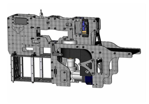
Secure the motor in the helicopter using four M3x12 cap head screws. There is a motor mount double plate provided for the outside of the frame as well.
