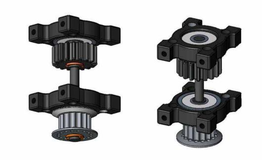
If you are building the budget series of bat helicopters, your counter gear assembly will look like this. It is assembled the same way as the regular bat counter gear assembly except that this one will work off the top gear for the budget bat auto hub.
