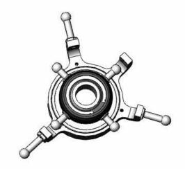
There are 3 M2 holes tapped in the lower ring of the Swashplate install the M2x4 Phillips head screws there. The lower outer ring of the Swashplate will get the M3x12 pivot balls, and the inner ring will get the M3x7 pivot balls. On the budget series bat you will add a straight pin to the 4<sup>th</sup> open position on the outer ring of the Swashplate.
