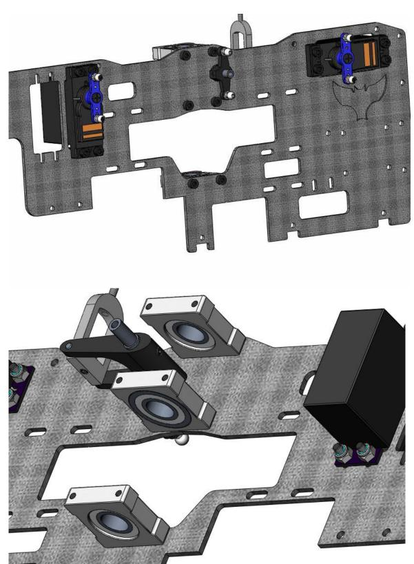
Attach the three main shaft bearing blocks to the upper frame. Be sure that the flanges for the two upper main shaft bearing blocks face each other. By flange, we mean the side of the bearing block
