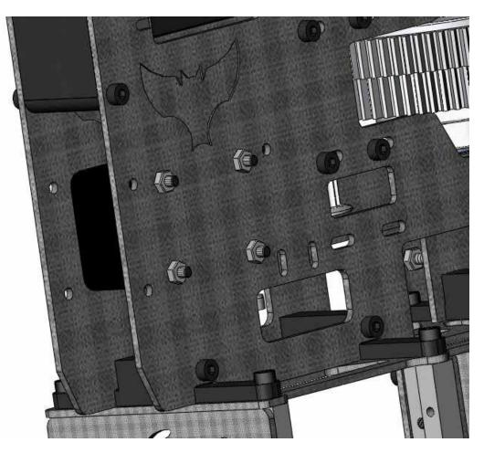
Now you can install the plastic boom holder blocks. Install the blocks with four M3x35 cap head screws and lock nuts.
