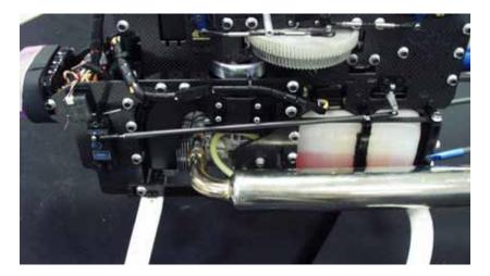
For the 70 and 90 sized helicopters you will need to cut a carbon rod to 210mm. Glue in the ends, and thread on a long ball end on each end. The ending rod should be ~263mm from ball to ball. You simply want to have your servo at straight up and down at neutral and then have the bell crank in the rear perpendicular to the side frame.
