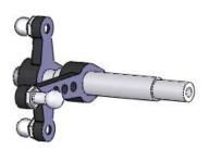
If you are building a budget series bat helicopter you will be using this style of elevator lever. You will assemble it onto the elevator shaft the same was as the other style with an M3x5 set screw. Install an M3x7 pivot ball stud into the arm.
