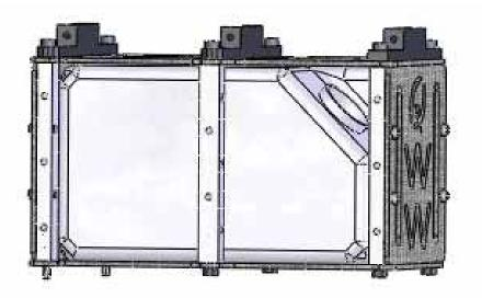
Install the M3x12 set screws into the rear two cross member-uprights. Attach the front and rear QWW stiffener plates with the M3x8 button head screws. It is a good idea to put a little foam tape or padding on either side of the fuel tank. This will add a little vibration isolation for the fuel tank.
