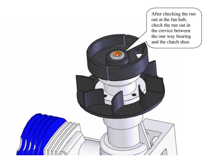
Attach the clutch shoe to the fan hub using two M3x8 cap head screws.
