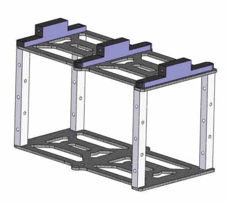
Assemble the fuel tank assembly as shown. You will have one shorter upper to lower mounting block and two longer ones. The longer ones go on the two rear sets of holes.
