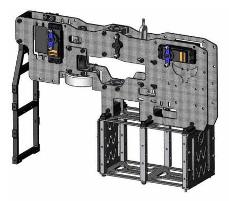
Attach the completed fuel tank assembly to the upper frame assembly with six M3x8 cap head screws.
