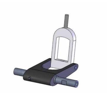
Attach the unit to the elevator control shaft using an M3x5 set screw. Be careful to install the shaft so the flat for the elevator bell crank comes out the same side you have your servo on. In our case we have is on the left side.
