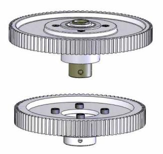
Now slide the lower main gear assembly onto the upper main gear assembly.
