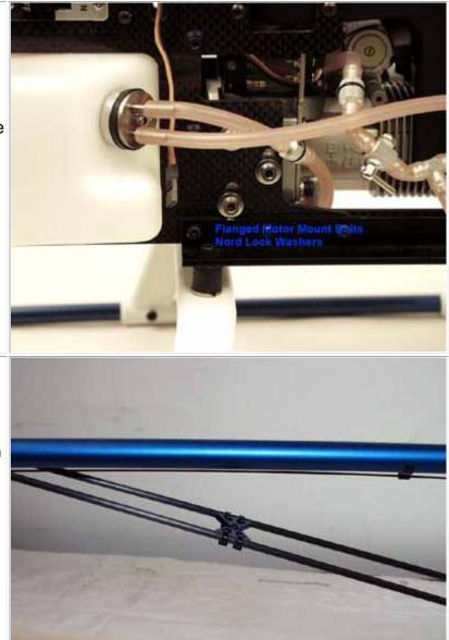
**Boom Brace -** The boom brace goes in between the dual boom supports and stiffens the whole systems up.
