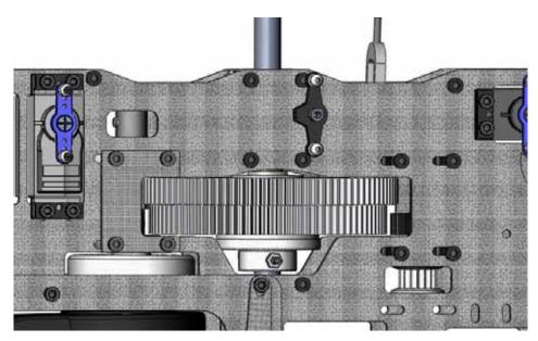
The lower main shaft bearing is vertically slotted so that you can adjust the height of the main gear to get the positioning perfect.
