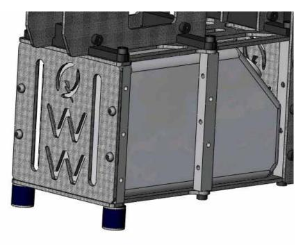
Attach two landing gear dampeners to the fuel tank assembly. Find two M3x12 set screws and install them into the landing gear dampeners using Loctite. Next, thread them into the rear fuel tank cross members.
