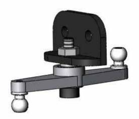
Attach two shim balls to the bell crank assembly with two M2x10 Philips head screws.
