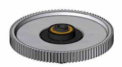
This is how it will end up looking from the top side. You will Slide the main shaft into the auto rotation hub in the same way as detailed earlier. Attach the autorotation hub to the main shaft using an M3x16 cap head screw and M3 Locknut.
