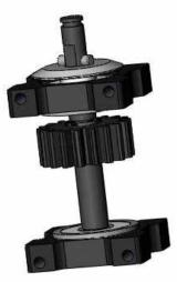
Now, slide the pulley gear side plate onto the counter gear shaft and slide through the pulley gear lock pin.
