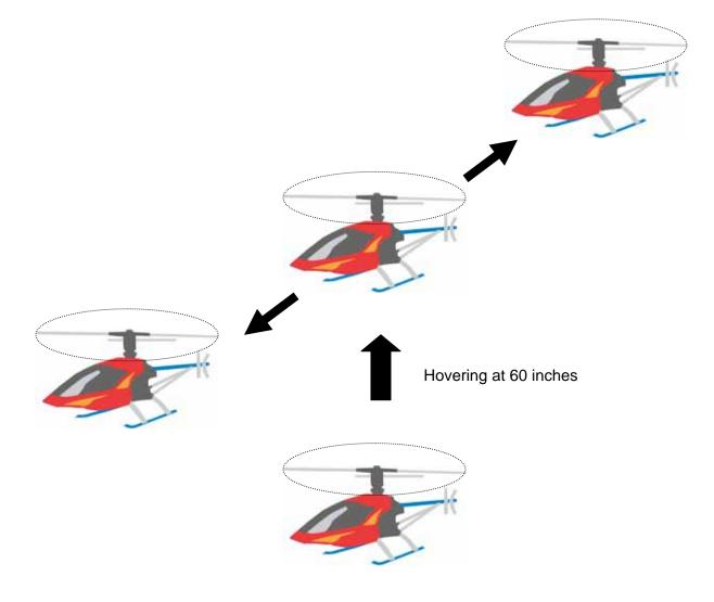
(b) Once you have been comfortable with all the movements and controls in the previous step, start using some tail rotor control to make the helicopter point slightly to the left or right as you fly it to the left or right. Keep practicing the figure-eight path as shown below, you will master all basic control movements of a helicopter.
