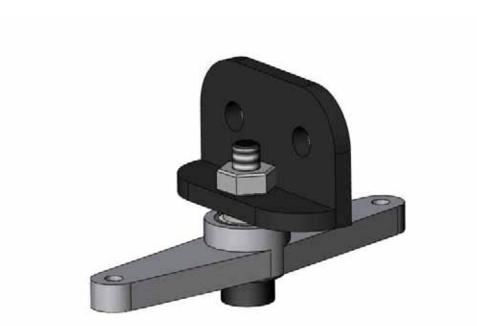
Locate your rudder bell crank mount and attach the Bell crank assembly with an M3 Locknut.
