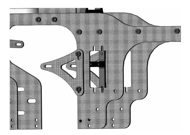
Now install the front fan shroud mounts. Use two M3x10 cap head screws for each. Leave these a bit loose as well until we install the fan shroud.
