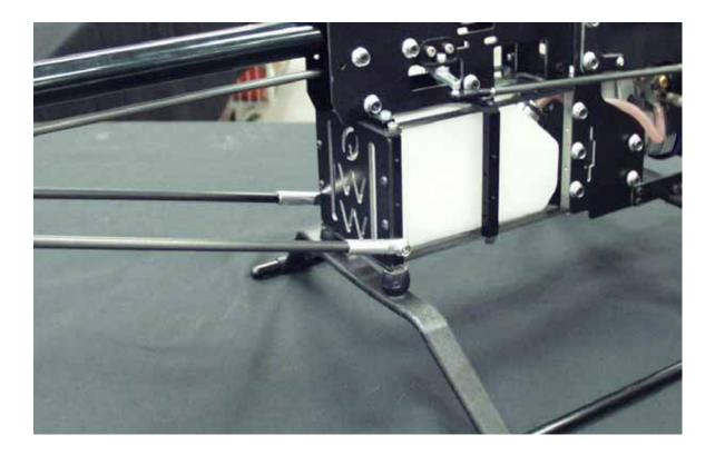
The pro series comes with carbon boom supports with aluminum ends. The Sport and Budget series come with fiberglass composite rods and plastic ends. Either one is assembled the same way. Cut the rod to length using a dremel cutoff wheel or something similar that won't split the rod. You just want the rod to be long enough that it won't allow the tail blades to hit the horizontal fin. Shorter is ok. Once they are cut to length glue the ends on with either epoxy or jb weld.
