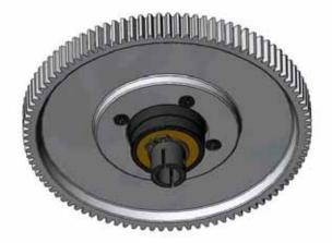
If you are building a budget bat you will have an autorotation assembly that will look like this. The gear slides up from the bottom and attached with (4) M3x6 Flat Head Screws.
