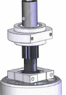
With the start shaft pushed all the way into the clutch bell attach the start coupler with an M4x4 set screw. When assembling this for the 70 or 90 clutch bells, you will use three 5x7x2 spacers between the clutch bell bearing block and the start coupler.
