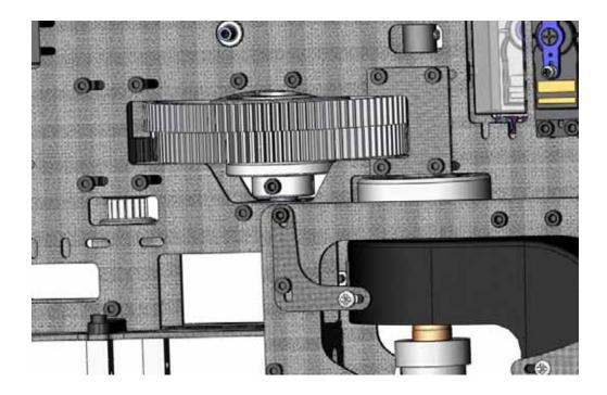
Next, you will slide your main shaft through the main gear hub assembly. The end with the longer distance to the hole goes in first. It will be the end going in first. Attach the main gear assembly using an M3x30 cap head screw and an M3 Locknut.
