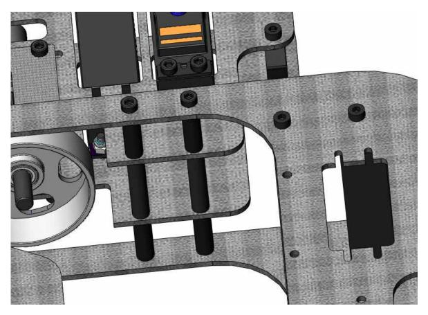
Locate two 26mm cross members. Remember to Loctite all screws and screw the outer spacers into the inserted 26mm cross members in the frame.
