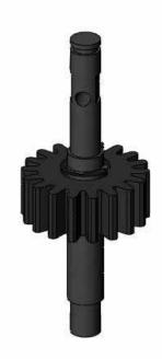
Install the M4 E-Clip into the groove to secure the counter gear.
