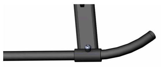
Secure the landing gear skids with (4) M2.5x6 self tapping screws.
