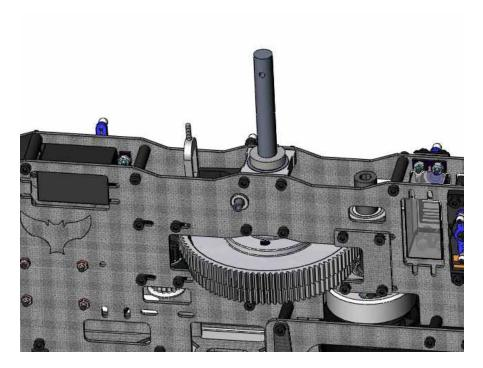
Slide the main shaft collar onto the main shaft. While pulling up on the main shaft to remove any play and tighten the collar with the supplied M2.5x8 cap head screw.
