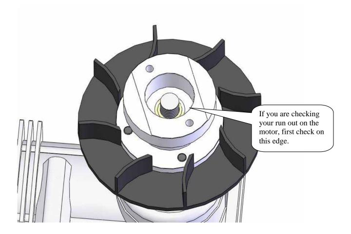
Slide the second smaller conical collet down onto the crank shaft. The tapered side goes down into the cavity. Secure the fan hub with the prop nut that is included with the motor. Note: It is important to use a Dial Indicator to check the run out of the Engine Assembly. Most of the vibration problems come from this. The run out should be no more than 0.004 inch (0.10 mm).
