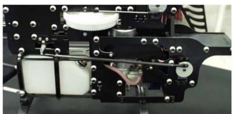
For the 50 sized helicopters you will need a carbon rod cut to 200mm. Glue in the ends, and thread on a long ball end on each end. The ending rod should be ~250mm from ball to ball. You simply want to have your servo at straight up and down at neutral and then have the bell crank in the rear perpendicular to the side frame.
