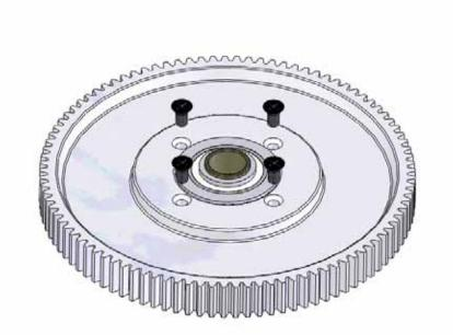
Attach the upper 97T main gear to the auto rotation hub using (4) M3x6 flat head screws. When you install the screws on both gears, tighten the screws in a cross wise fashion to get equal pressure on the gear and ensure that the gears sit flush onto their hubs.
