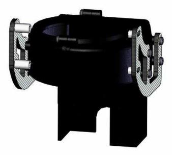
Locate the two fan shroud mounts. They will be in your frame bag. Attach them to either side using 4 M2.6x10 self tapping screws. On the Right side of the helicopter when you attach the assembly to the helicopter you will use 2 3x5x3 spacers. On the other side, you will use 2 9mm spacers.
