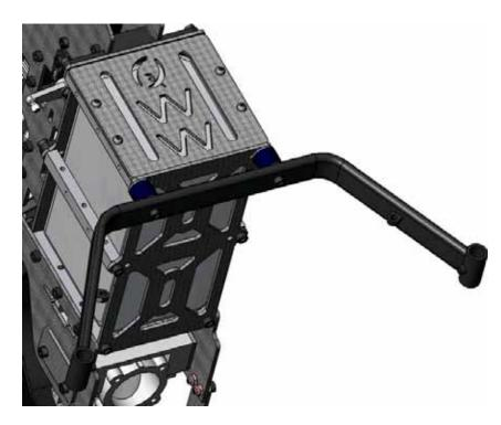
Attach the landing gear to the dampeners as shown. Use two M3x10 cap head screws. You will need to drill two M3 or 1/8" holes in the plastic to mount the landing gear. It is 70mm from hole to hole on the rear landing gear and 60 on the front one. **TIP:** One method for aligning the holes properly is to take a piece of masking tape and put it on the mount for the helicopter. Mark the holes with a magic marker or pen and then transfer the tape to the landing gear and drill the holes.
