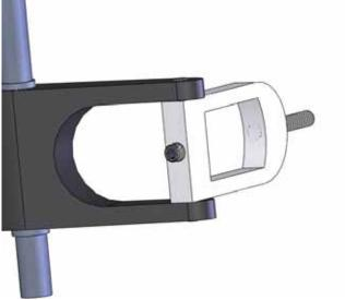
Install an M3x5 set screw into the bottom of the elevator control unit to secure the pin.
