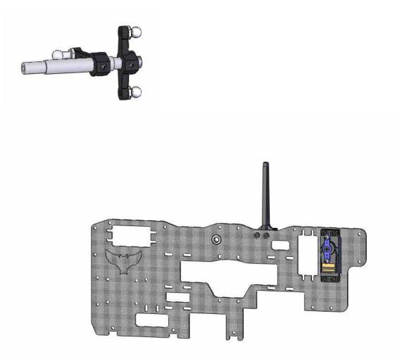
This step is only for the budget series helicopters. Install the Swashplate anti-rotation guide to the main frame using 2 M3x8 cap head bolts. You will install two on the opposite side when the other frame half is attached.
