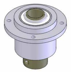
Locate your auto rotation sleeve and spacer. You will slide your auto rotation sleeve into your hub and slide the spacer on the top. You can leave the spacer off until you are ready to install the unit into the helicopter.
