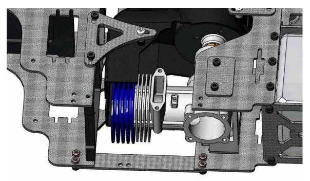
Attach the landing gear mounting plate to the engine frame with five M3x8 cap head screws and four lock nuts.
