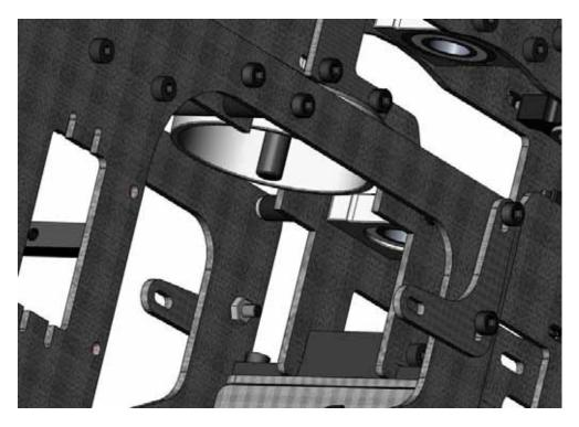
Next we will attach our rear fan shroud mounts. For the upper hole we will use an M3x25 cap head screw. Remove the M3x8 cap head screw in the lower main shaft bearing block. Install the new screw through the fan shroud mount, then through the engine frame, then through an 18mm spacer, and finally into the bearing block. You can leave this sort of loose for now, until the fan shroud is installed and adjusted. The lower screw is an M3x8 cap head screw and a lock nut.
