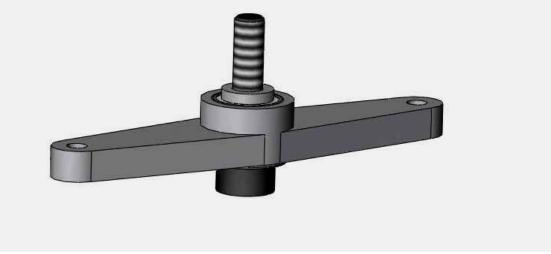
Insert an M3x14 cap head screw as shown. Slide a 3x5x3 spacer onto the screw,
