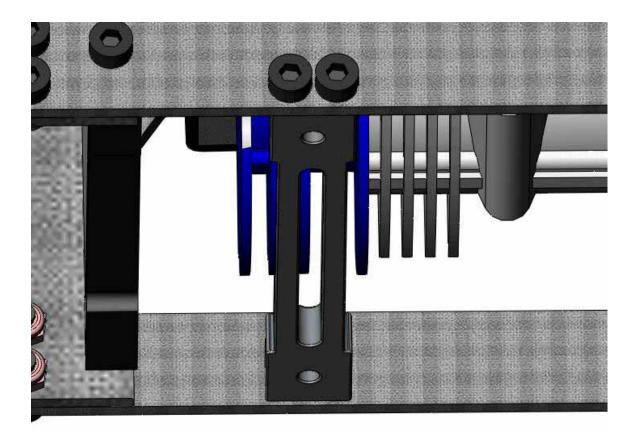
Attach the landing gear mount with four M3x8 cap head screws.
