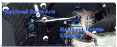
Machined Servo arm set - The aluminum servo arms provide a lot of extra strength to the control system. When you use plastic arms they flex and can produce interactions (Interaction is when you put a specific command into the helicopter but the helicopter doesn't produce the desired output.), but the aluminum arms don't flex at all.
