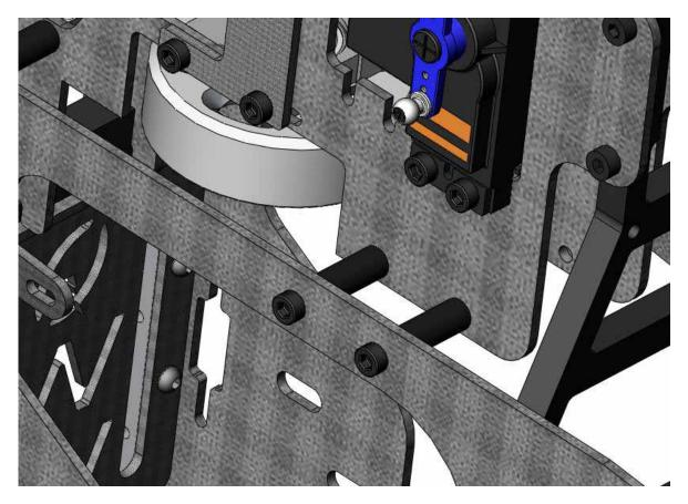
Now we can install the two frame cross members. First, gather four M3x25 cap head screws and four 18mm frame spacers. Slide the bolt through the frame slide an 18mm spacer onto the bolt and slide the bolt through the hole in the main frame assembly.
