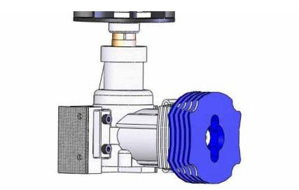
Attach the motor mount to the motor using four M3x10 cap head screws. Using Nord-lock washers are a nice accessory to use here. The motor mount is not symmetric. The end that has the further distance to the end from the screw hole will down as shown in the picture.
