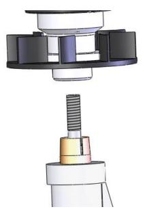
Slide the fan hub assembly onto the crank shaft.
