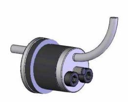
You will only need one line for fuel tank pressure so the other two holes in the stopper can be plugged off. This can be done with a few M3 bolts. When the stopper is tighten it will seal around the bolts.
