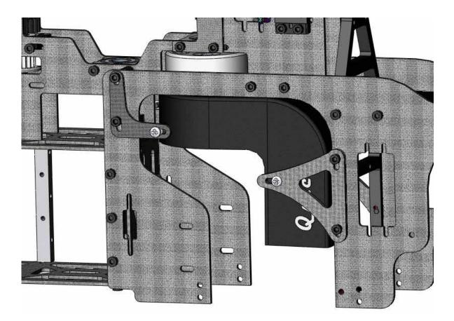
Install the fan shroud as shown. Attach the fan shroud using (4) M2.5x10 self tapping screws. Use a 3x6x5mm spacer between each mount and the fan shroud.
