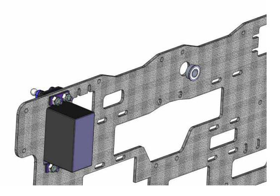
Note: The holes on the frames are designed for "push-fit" feature. Sometime you may have to use a round "rat tail file" before pushing the bearings in. The bearing flange mates against the inside of the frame. The flange is set on the inside of the frames. The elevator shaft will hold the bearing in place.
