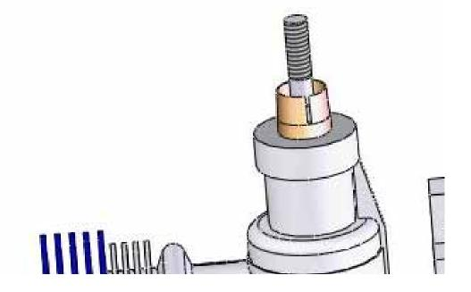
Next, install the engine collets. First is the one that just looks like a spacer/washer. Then the larger conical collet goes on.
