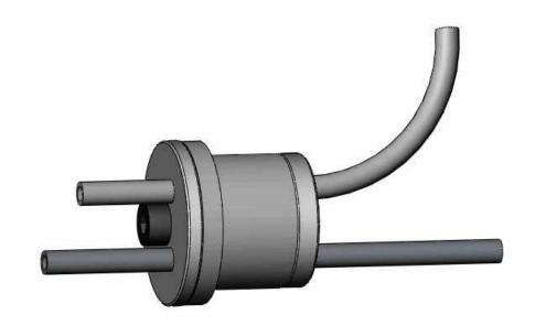
You can run your fuel tubing two ways. One is to use two tubes coming out of the fuel tank stopper. The one that curves upward will go for the fuel tank pressure line. The Other line will have the clunk hanging off of it.
