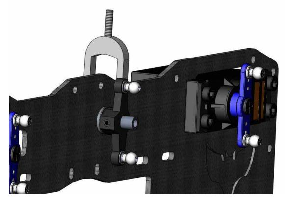
Install the elevator assembly into the bearing in the upper frame assembly and attach the outer elevator arm with an M3x5 set screw. Install two M3x4 pivot balls into the elevator arm.
