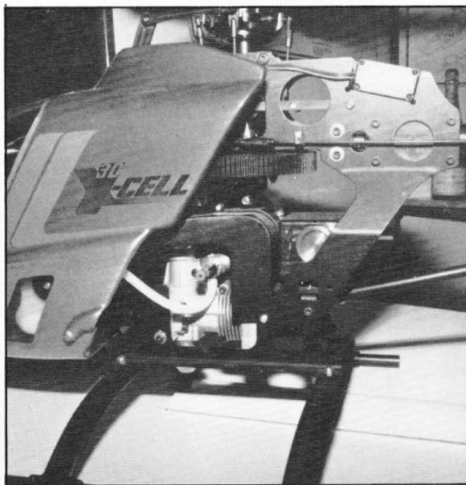
The new M.A.S. X-Cell 30. This machine was on the Modtec stand at Sandown. Points of interest to the writer included a top and bottom cone start courtesy of an OS32 with integral rear cone. Also note the rearward gyro mount and the mini quiet pipe. This small M/C will do to the 28/32 market what the 50/60 has done to the fullsize.
