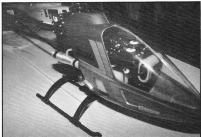
The new M.A.S. X-Cell 30. This machine was on the Modtec stand at Sandown. Points of interest to the writer included a top and bottom cone start courtesy of an OS32 with integral rear cone. Also note the rearward gyro mount and the mini quiet pipe. This small M/C will do to the 28/32 market what the 50/60 has done to the fullsize.
