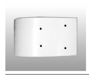
Begin the gasoline tank assembly by locating the gasoline tank holding trays. Inspect the bottom of the tray and locate four hole location marks. Drill all four marks with a 3 mm (1/8") drill bit. Repeat this process on the second tray.
