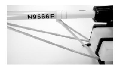
through the longer strut then the shorter strut and through the hole in the side frames and secure with one 3mm Locknut on the inside. Once both sets of struts are tightened on the lower side frames, align the struts and tighten the ends on the tail boom.
