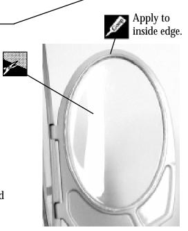
On the bottom of the canopy there are two small indentations. Drill two 3mm (1/8 inch) hole at these marks. Locate the Inside Canopy Mount [HI3129]. Note that this mount is designed to fit one direction, the wider end should face towards the helicopter. Attach the mount to the inside of the cabin utilizing two 3x10 self tapping washer head screws.
