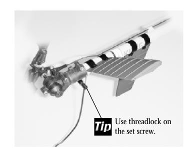
At Step 37, locate the two sets of tail boom supports (one long set and one short set). Loosely attach one end of each of the short boom supports to the strut mount closest to the front using one 3x16 Socket Cap Screw with 3mm Locknut. Similarly, loosely attach the longest set of tail boom support rods the rear most strut mount using one 3x16 Socket Cap Screw with 3mm Locknut. Bring the two struts together, insert one 3x16mm Socket Cap Screw
