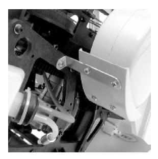
The tail boom, tail pushrod guides and tail boom supports should be painted at this time before assembly. Remember that the pushrod guides may need to have the inside holes sanded slightly larger to fit the painted tail boom.
