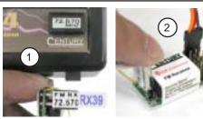
2. Note that all electronics plug into the receiver with the wires as pictured (orange wire faces receiver label). Follow the diagram for each electronic connection. Once the electronics system is connected and the transmitter is turned on, follow this step-by-step process to check your equipment.
