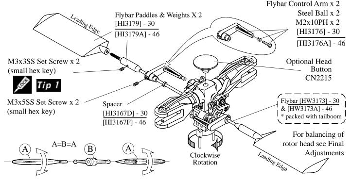
Align each paddle 'A' to be parallel with the flybar control arms 'B'. This is made very simple with the optional pitch and paddle gauge CN2026
