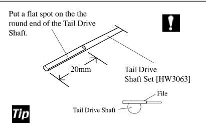
A flat file is the ideal tool for the job, alternately careful use of a Dremel Moto Tool will work. It is important that the flat be at least 1/4 of the diameter but no more than 1/3 to avoid weakening the material.
