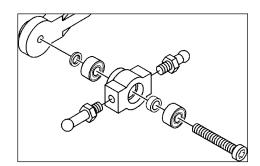
Tip 4: For machine screws, tap the hole ahead of time using the screw being careful not to strip out the threads as in some locations the plastic hole has a bottom. Finally assemble the parts for that step. Remember that machine screws can load bearing if overtighten. In these cases carefully tighten the machine screw then back of 1/16th of a turn.
