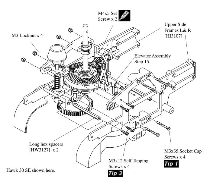
Note : The gear mesh between the main gear and the tail transmission output shaft should be a snug fit and will become smooth after a few flights, this is the normal wear in process.
