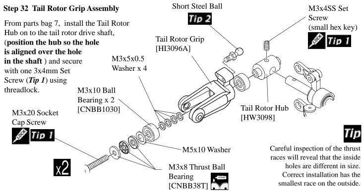
Install one short steel ball into the upper right
