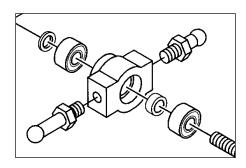
Tip 2: In many locations in the assembly steel balls need to be threaded into plastic parts. To make this an easier task, use an available 3x16mm socket cap screw with a hex key and tap the threads ahead of time. When tightening the steel ball, use an open ended metric 5 wrench which will match the hex exactly and not damage the ball. Standard pliers can easily slip and scratch the surface of the ball which will prematurely wear the plastic ball links.
