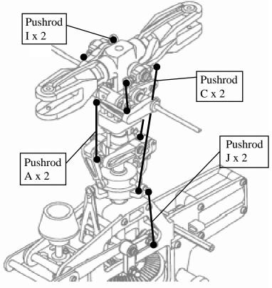
Step 44 Rotor Head Linkage & Elevator Linkage
