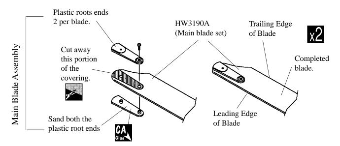
Note: The plastic blade grips have a top and a bottom which are different when viewed from the large end. Test fit the parts to be sure that the total thickness of the blades are 12mm.
