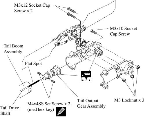
Apply red locktite to the drive shaft end **only** and insert into the gearbox input shaft. Do not use on set screws, only bond the wire shaft to the input shaft. Tighten the set screws equally to make sure the wire and input shaft spin on the same center, especially when making field adjustments through the hole in the gearbox ( any clicking from the tail box indicates this problem.)
