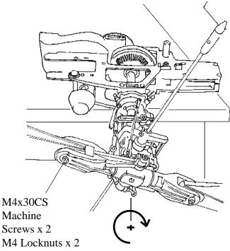
When attaching the main blades, the direction of rotation is clockwise, when looking on top of the helicopter.
