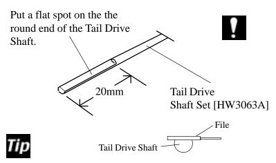
A flat file is the ideal tool for the job, alternately careful use of a Dremel Moto Tool will work. It is important that the flat be at least 1/4 of the diameter but no more than 1/3 to avoid weakening the material.
