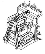
Using the foam rubber, wrap the battery pack, receiver and gyro controller(mechanical type) separately, allowing wires to be collected and tied together. Using two elastics looped through the front of the top servo tray, secure the components to the two hooks on the lower servo tray. Depending on your equipment, the gyro controller and switch can be mounted on the provided bracket.
