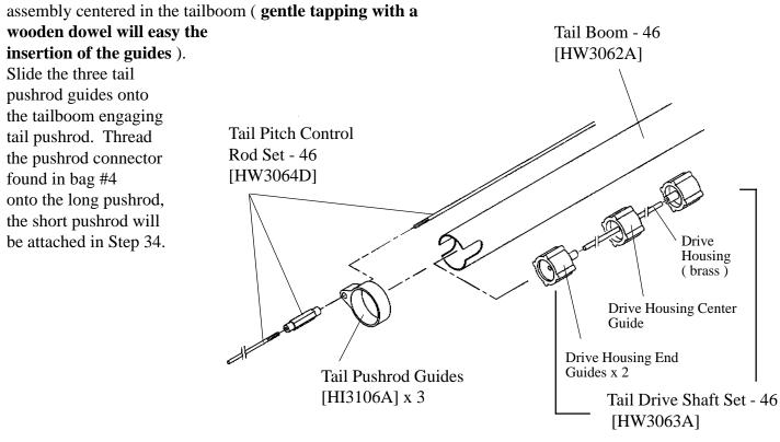
Make sure the brass tubing is glued to the internal guides for the tail boom. Also, after radio set up is complete glue the pushrod guides using a single drop of Zap Ca. One drop will stop the pushrod from binding and still be able to remove them later.
