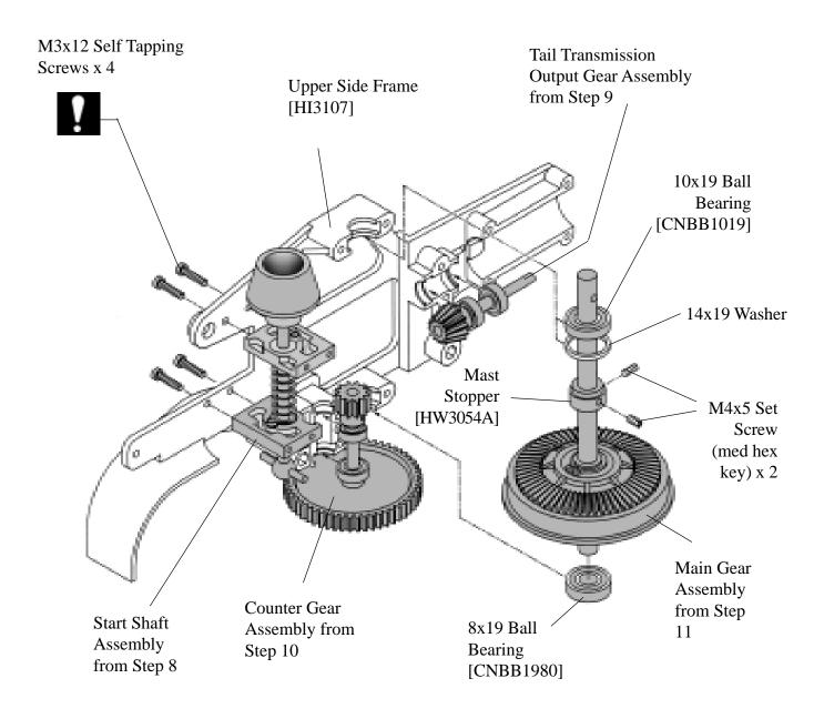
Note 1: Be careful when tightening the eight 3x12mm self tapping screws into the start shaft block assemblies as excessive force will strip out the plastic holes.
