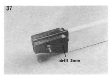
Cyano-glu) into the Blade Joiner (CO.2) to minimise play, when doing this, check the slot in the Rotor Head is 90 degrees to the Blade Joiner, Fig 33.
