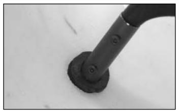
14. Secure the Aluminum Strut and Brace with 2.6x14mm Socket Screws. Hint: Install the left Aluminum Strut Assembly and Brace first (Left side is the side of the fuselage with Optical Missile Sight). Pull the brace out and secure the socket screws then push it back and pull the right side out then install the right aluminum strut assembly.
