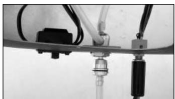
**32.** You will have to install the remote glow plug adaptor (TTR3803). With the opening for engine cooling located at the bottom of the engine, you can either use the glow starter from the opening or install a Built in Glow Plug Extension Wire (TTR2174) and secure the connector on the fuselage for easy glow ignition. Also suggested is the use of Precision Fueler Valve (TTR1115) which is very convenient for both re-fueling or de-fueling and could filer the fuel when fueling.
