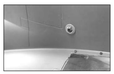
**26**.Secure the fuselage with 4x10mm Button Head Screw and M4 Washer as shown.
