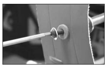
24. Remove the damper temporarily and insert the Silicon Grommet from the inside fuselage then re-install the damper again. Note the bigger diameter side should be facing the Damper. Secure the fuselage with 4x10mm Button Head Screw and M4 Washer. Do the same procedure at the other side.
