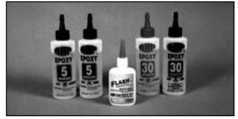
Adhesives - You will need two types of adhesives for the MD-500 - Epoxy and Instant (cyanoacrylate) adhesives. We recommend that you purchase both 5minute and 30-minute epoxy to cut down on assembly time, but you can get by with only 30-minute epoxy if time is not important. You will also need a small bottle of both "Thick" and "Thin" instant CA adhesive.
