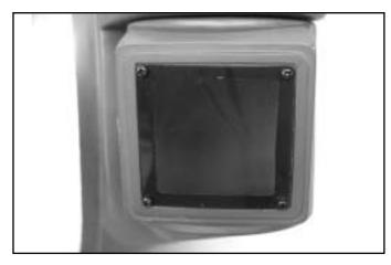
**3.** Locate the Sight Lens, position it in place, then drill 1/16" (1.5mm) holes at the four corners. Secure the lens in place with four 2x5mm Wood Screws.
