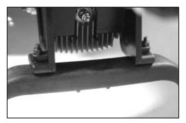
**20**.Secure the helicopter onto the landing brace with four 3x30mm Socket Screws and M3 Locknuts. Secure the rear brace first then the front.
