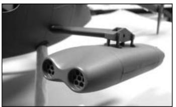
**30.** Locate the Joiner and insert it into the pod retainer, next trial fit the missile pod assembly onto the wing. Make sure two missile pod are angled just right, if not then trim it until it will. Remove the missile pod assembly then apply epoxy at the joint area in the wing then secure the wing with 3x25mm Wood Screw. Make sure again that the two missile pods are at same angle.
