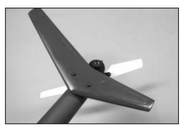
**21**.Secure the Vertical Fin in place with two 3x40 Socket Screws, two M3 Washers and two M3 Locknuts.
