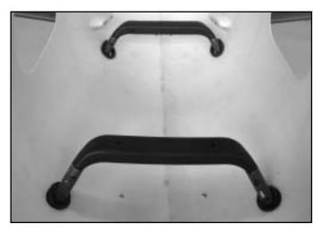
**13**. Remove the landing skid assembly from Heli. Remove the brace from the aluminum strut. Do not remove the strut and skid pipe as they are already adjusted and secured. Apply masking tape on the strut that is going to make contact with the fuselage, since the masking tape will protect the paint from scratching. Place the brace on the fuselage and install the strut and skid pipe onto the brace. You may apply Vaseline on rubber ring to increase the lubrication for easier installation.
