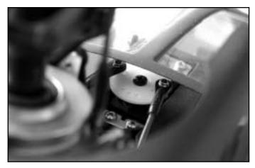
16. Trial sit on the landing skid assembly. For Raptor owner, position the Front Windshield in place and check if the ball links on aileron servo horn contacts the front windshield when it is in maximum positive pitch. Lower the Raptor by enlarging the landing strut opening to the fuselage center liner if the servo horn contacts the windshield. It might be necessary to try several times before obtaining a desirable result.
