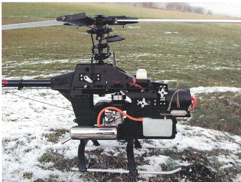
Large fuel tank gives good flight times. Paddles weight is adjustable by the amount of lead you insert, the large area gives good control response, while more weight will make it more stable. Sturdy undercarriage is mounted on dampers which will help absorb landing shocks.
