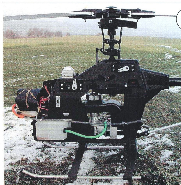
Servo tray is quite short and extra weight was needed to bring the C of G to the mast. The on/off switch is easily reached with the canopy in place.
