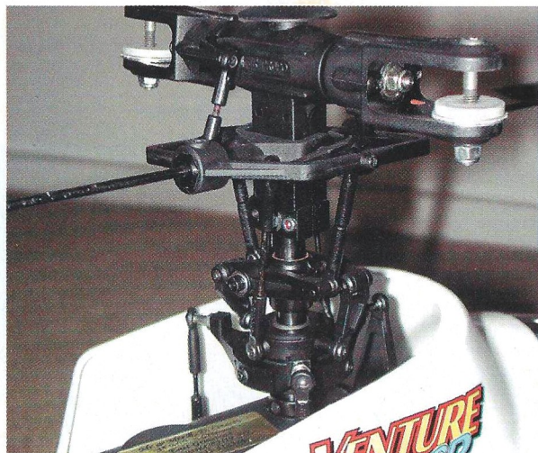
Flybar carrier has Hex inserts to transfer Hiller inputs to the 3 mm flybar. The mixer base has Oilite bushings. Swashplate is GRP with M3 set screws to pre-load the bearing if needed. Mixer arms have 2 positions for the output ball links - use inner hole for softer controls.
