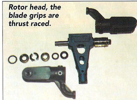
Two ball races support the tail blade grips.
