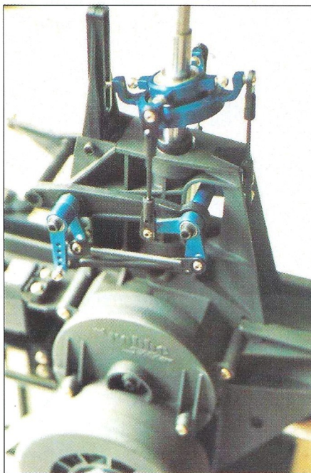
Collective and cyclic levers. The fore/aft lever is longer than the roll lever and the roll swashplate link can collide with its double link: See text for details.
