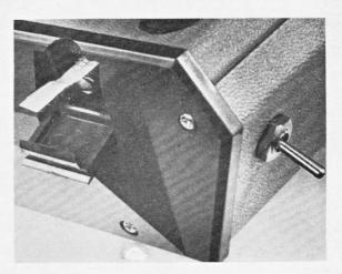
Transmitter P.C. board is quite sparse. Control stick mode is easily altered by simply transposing a ratchet brake from one stick assembly to the other – not necessary to remove centring springs, but to achieve this, the case sides have to be removed. Plug-in crystal is accessible through small hatch in case side – a neat feature. Six sets of crystals are provided, plus frequency penants.
