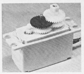
Futaba FD15M is one of the smallest in production. Features rotary output. Unusual sloping end of case permits the end of a wooden push rod to come nearer to the rotary output disc, thus shortening the wire push-rod end and achieving a more whip-free linkage to the control surface. Gear train features deep output gear to withstand shock loads. Servo are provided with unit.
