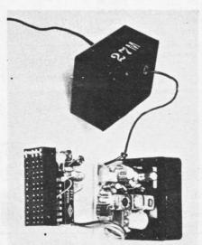
Left: very small receiver is laid out on two P.C. boards; one contains the IF section the other the IC decoder and block connector. Short lengths of lead interconnect the two boards. Right: transmitter is tidily arranged. The RF section to the RH side of the board is a separate plug-in unit - can be exchanged for alternative frequency bands for overseas trips.
