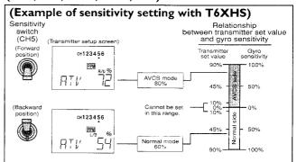
The figure above uses the CH5 ATV function and is an example of switching to hovering (AVCS mode) in the switch forward position and to idle up (normal gyro mode) in the backward position) and setting the sensitivity of each mode to 80% and 60%, respectively.
