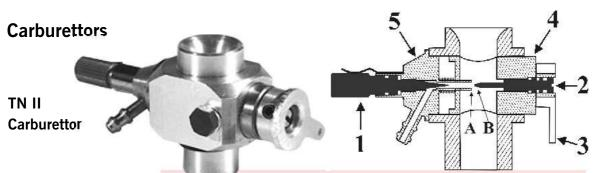
1 High-speed needle 2 Idle needle 3 Throttle arm **4** Throttle barrel 5 Spraybar
