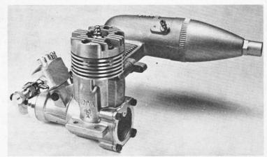
Shaft end threaded M7  $\times$  1.0 for prop nut.
