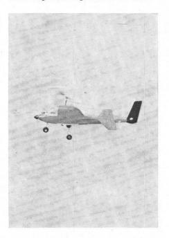
Action sequence of first flight, back in May 1970, when pictures were taken 'just in case'. Note that this prototype has much less side area than the latest version shown on the plans. 'Elevator' control is used to alter the rotor incidence and directional control is applied via 'ailerons' on tailplane. Rudder is normal.
