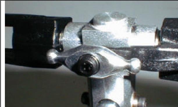
Attach each hiller arm to the blade grip using an M3x10 cap head screw. Put the bolt through the hiller arm and put a 3x5x1 spacer on the bolt next, and screw it into the blade grip.
