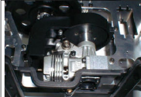
Slide the engine up into place and secure it using (4) M3x6 cap head screws.
