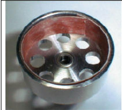
Locate the lining and cut it to 98mm. Glue this in place with JB Weld. The best way we to hold the clutch liner to the bell is to wrap the clutch with a few rounds of electrical tape and slide that into the bell.
