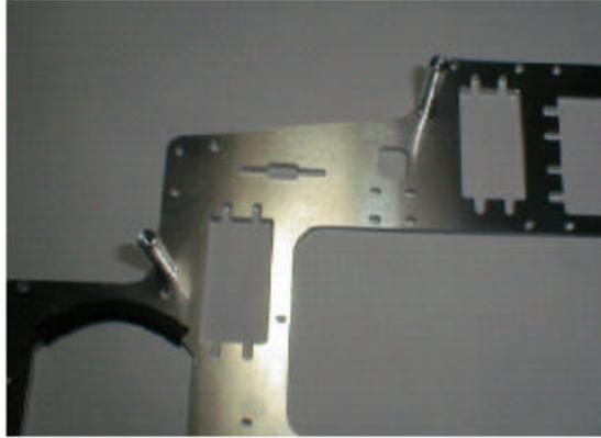
Slide two frame halves over fuel tank with canopy mounts facing outward. The fuel tank is on the front of the helicopter, so looking from behind the helicopter the open hole on the tank goes out to the left.
