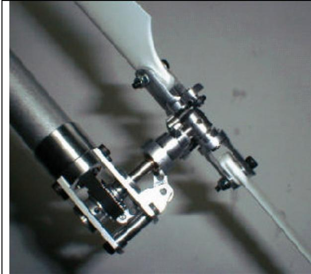
Attach a tail blade to each grip using (2) tail blade spacers, an M3x20 cap head bolt, and an M3 locknut.
