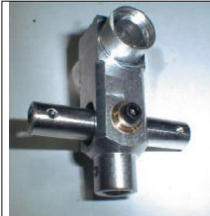
Locate the head block, seesaw, seesaw collars, and (2) M3x8 cap head screws. Slide the seesaw into the opening on the head block. Slide a seesaw collar into each of the bushings on the head block. Secure the seesaw using the (2) M3x8 cap head screws.
