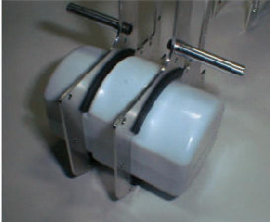
Install upper and lower main shaft bearing blocks using (8) M3x6 cap head screws. Note: Be sure that on the upper bearing block the open half faces up. The lower block the open face should be down.
