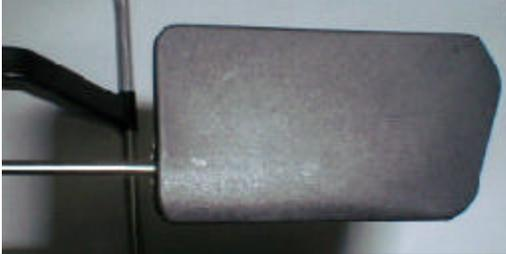
Screw each paddle onto the flybar 25mm. Be sure the paddles are parallel with each other. Also the paddles should be inline/parallel with the flybar control arms.
