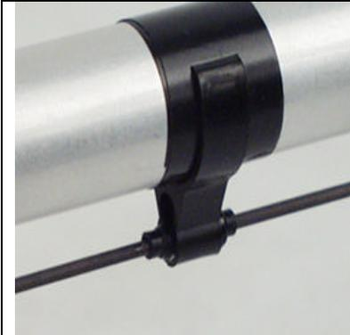
Assemble the push rod guides. There are three pieces the main clip and two inner sleeves. Simply slide the two sleeves into each other and then into the main clip and glue. Putting electrical tape onto the boom before gluing is good, so it is possible to reuse the clip later. (HHI2900 – Rod Guides)
