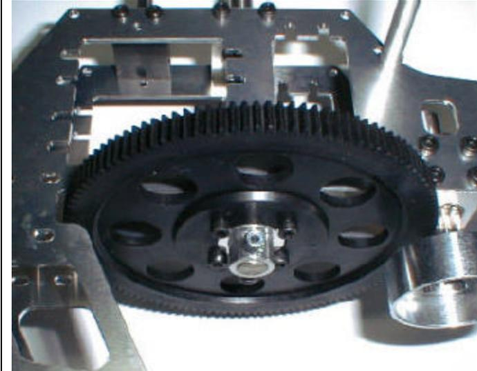
Slide the main shaft through the two main shaft bearing blocks. The end with the hole closer to the end should go down through the blocks from the top side first. The main shaft will slide through the main gear assembly. Lock the bolt in place using a M3x18 and a M3 Locknut
