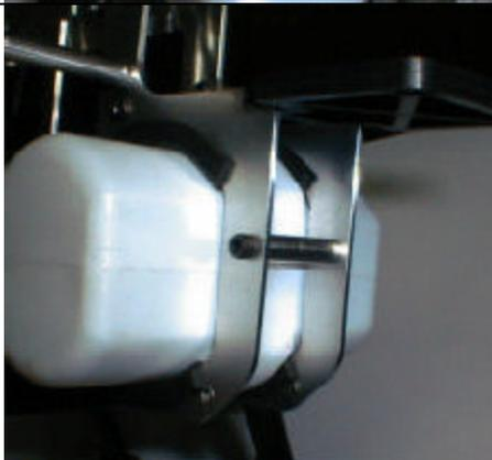
Install the anti-rotation guide using (4) M3x10 self tapping screws.
