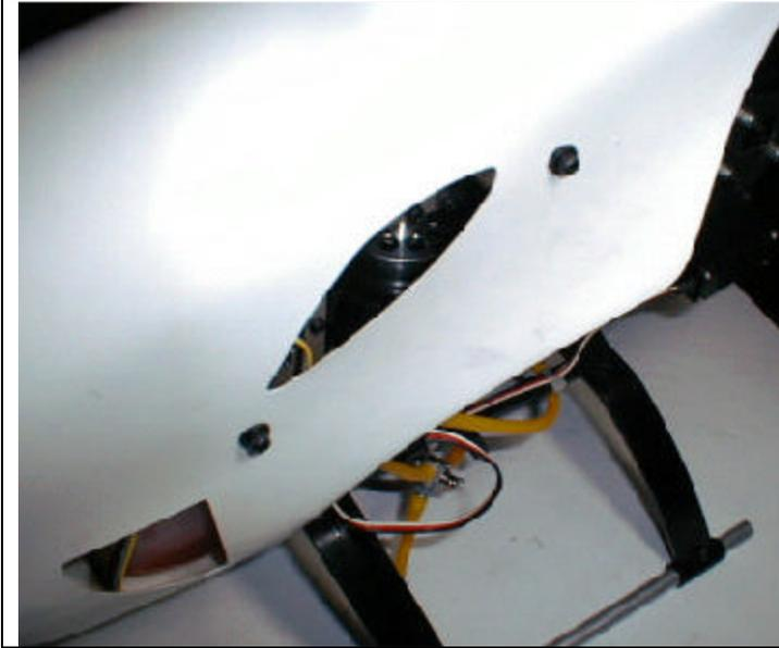
Place the canopy where you like, mark the holes for the canopy standoffs. Use a 1/4" drill bit. Place the grommets in the holes and secure the canopy to the helicopter using (4) M3x14 cap head screws.
