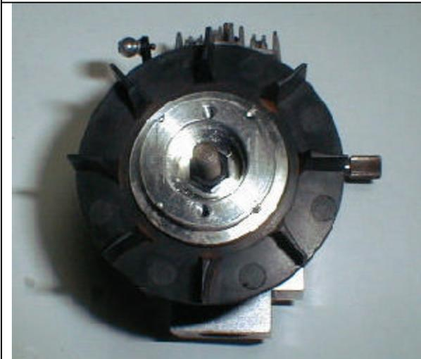
Install the fan hub onto the crank shaft and secure it in place using the nut provided with the engine. Be sure to use red threadlocker to ensure the nut does not come loose.
