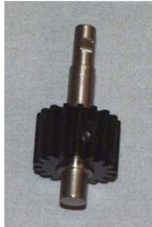
The Counter Gear Shaft pictured on the left illustrates the reduced portion of the shaft. make sure the pulley is fastened to the flat shown in this picture.
