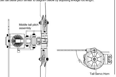
Next set the direction of the transmitter rudder function when you move the rudder stick to the right, the ball on the tail rotor servo horn should travel toward the rear of the helicopter. Use the transmitter reversing function to correct this.
