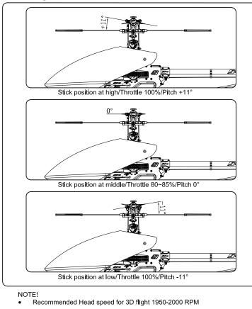
! Caution: For safety of flight and helicopter structure. Main rotor speed should not Exceed 2100 RPM or maximum RPM set by rotor blade manufacturer.
