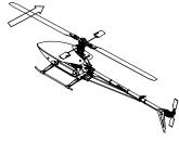
To test the gyro direction, move the nose of the helicopter right.
