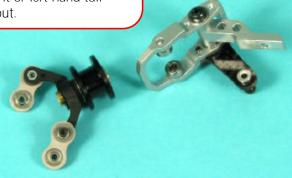
New Design heavy duty T/R blade holders ensure smooth tail response
