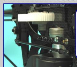
New Right Hand T/R output improves tail rotor control response for precision hovering and also improves model tracking during rolling maneuvers. The servo and primary control linkage are the proven Fury design. Front bellcrank now proides a 1:1 mixing ratio
