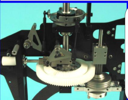
All new CNC milled graphite frames offer improved servo positioning.
