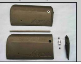
All New Pro-3 Fly bar Paddles. Easily assembled and allow for easy weight adjustment at any time. Thicker airfoil ensures smooth cyclic response. Weight ranges from 38 gms to 65 gms.
