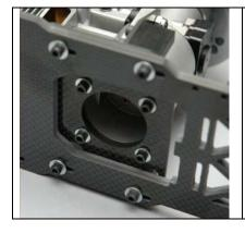
Slightly loosen the four bolts that attach the engine mount plate to the bottom plate so that the entire engine assembly can be repositioned in the slots on the bottom plate. Leave these bolts loose until the engine alignment is done in a later step
