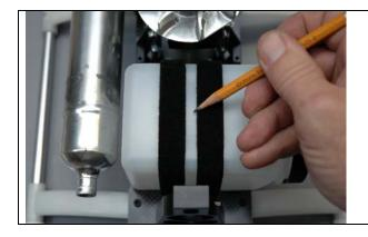
After positioning the fuel tank, use a pencil mark a spot on the top of the tank exactly between the two Velcro strips. Getting the exact side to side location correct is more important than getting the front to back position correct. Later you will install the fuel vent fitting here so you want to make sure it can clear the Velcro.
