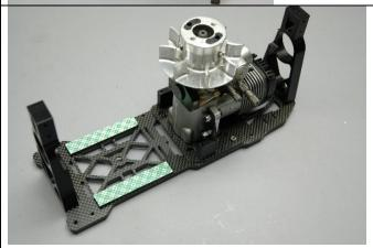
Select two #126-26 frame ladder support, four #0065 M3 x 12mm socket head bolts and four #0009 M3 washers.
