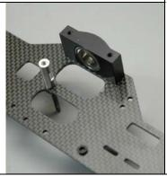
Select the double bearing main shaft mounting block removed from your original model and two #0061 M3 x 8mm socket head bolts.
