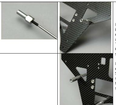
Insert one of the #0053-5 M3 x 16 threaded studs into the rudder bellcrank mounting post from your original model as shown after applying a small amount of red Loctite to the threads on the stud. Thread it in until  $\frac{1}{2}$  of the threads are inside the post. Carefully wipe any remaining visible Loctite off of the stud threads and allow this to dry.
