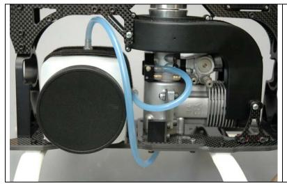
Plumb the fuel system as you normally would. The outlet on the top of the tank should be used as either the pressure outlet from the muffler, the pressure outlet from the engine (if it uses crankcase pressure) or the fuel overflow from the carburetor if you are using a pumped system.
