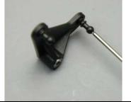
Select the two side bellcranks from your original model and remove the threaded balls. Select the four #0107 from Bag 2A. Apply a small amount of slow Cyanoacrylate glue to the threads on the ball and use a 1.5mm allen driver to insert the two threaded balls into each of the two bellcranks as shown in the photo.
