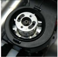
It is now time to mate the upper and lower frames. This will include pushing the clutch driver alignment ball and pins into the engine fan and dampers.
