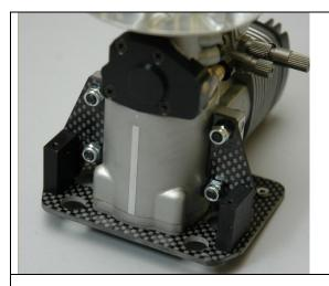
Select four #0080 M4 x 14mm bolts and four #0021 M4 locknuts
