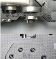
Select six #0061 M3 x 8mm socket head bolts and install as follows:
