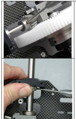
Now rotate the pinion gear again and remove the socket set screw that is against the t/r shaft flat. Apply a small amount of blue Loctite to the threads on this socket screw and reinstall it. Tighten against the flat on the t/r shaft. Now rotate the pinion a final time and fully tighten the remaining socket set screw
