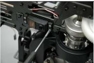
Insert the throttle servo into the frame position shown with the servo splined shaft towards the back of the model. Using the throttle servo mount bolts from your original model, apply a small amount of Loctite to the threads and tighten the servo into place. Follow your servo manufacturers instructions as to how tight these bolts should be
