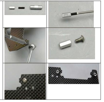
Select the four #125-12 frame channel spacers and four #0060-1 M3 x 6mm bolts.
