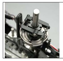
Select the washout assembly previously removed from your original model and slip it over the mainshaft.
