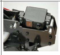
Select the elevator servo, four #0039-2 M2.5 x 16 Phillips head bolts, and two #575-3 servo blocks.
