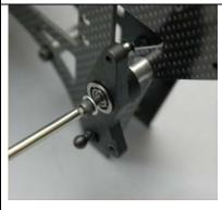
Select the t/r control bellcrank removed from your original model.
