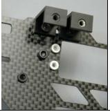
Select a #126-69 22mm spacer and a #0060-1 M3 x 6mm socket head bolt.
