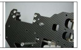
Select the #126-62 front doubler plate and lay it as shown on the outside of the right frame. Select two #0061 M3 x 8mm socket head bolts and one #0060-1 M3 x 6mm socket head bolt and insert as follows:
