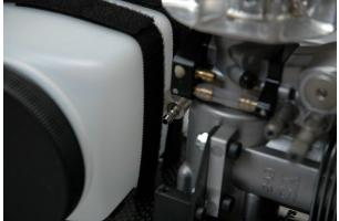
Tighten the two Velcro strips to firmly attach the tank to the bottom plate.
