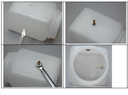
Use an x-acto blade or other sharp knife to remove any flashing on the holes. Be careful not to cut or damage the tank.
