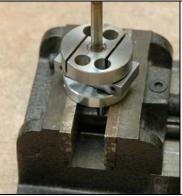
Using the fan tool supplied in your original kit, insert Two 4mm bolts (at least 20mm long) and nuts through the two slots in the tool so that they both protrude from the same side of the tool (see picture).
