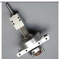
Insert the complete clutch/driver assembly into the assembled upper main frames as shown in the photo. Align the holes on the upper and lower bearing blocks as shown.
