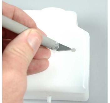
Remove any flashing from the drilled holes using a razor knife. Be careful to not enlarge the holes
