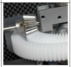
Using two fingers push the constant drive assembly/crown gear firmly up against the pinion gear while holding the lower retaining collar up against the middle mainshaft bearing. Tighten the lower retaining collar. Do not overtighten these bolts as the collar can crack. The correct way to tighten these bolts is to tighten until the socket head contacts the retaining collar and then tighten an additional ¼ turn.
