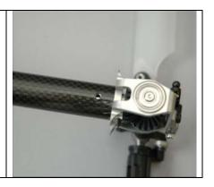
Select the right hand t/r mount clamp, which is also the vertical fin mount, and place it over the rear of the tail boom and against the t/r transmission as shown. When you aligned the t/r transmission and boom holes previously, it was to allow the M3 x 8 bolt on the side of the boom clamps to thread into the transmission.
