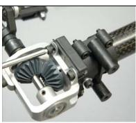
Insert four M3 x 10 bolts into the t/r mount clamp half bolt bosses as shown. Thread them in until the bolts are flush with the bottom face of the clamp.
