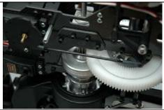
Snap the control rod onto the ball on the servo wheel and onto the control bellcrank on the left side of the frame.
