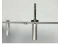
Select the #0169 bellcrank stud and insert it on the outside of the left frame in the hole at the center of top of the frame as shown. Apply a small amount of Thread lock on the stud threads and thread on one of #115-20 round frame spacers. Use appropriate tools fully tighten this. Orient the square part of the stud to as shown to so that it does not extend into the open cavities
