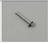
The first clip needs to be pushed over the pin to the approximate position shown. An easy way to do this is to drill a small hole in a block of wood (#30 drill), place the clip/pin over the hole and lightly tap the pin through the clip into the hole. If you tap it in too far, the clip can be adjusted using a pair of pliers.
