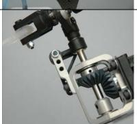
Now insert the pushrod from the front of the helicopter, through the previously installed push rod guide, so that the end with the brass tube is towards the front of the helicopter.
