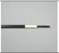
Using a round file, roughen up the inside of the remaining end of the t/r pushrod, about 1" inside.
