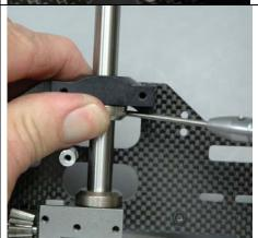
Now rotate the pinion gear again and remove the socket set screw that is against the t/r shaft flat. Apply a small amount of blue Thread lock to the threads on this socket screw and reinstall it. Tighten against the flat on the t/r shaft. Now rotate the pinion a final time and fully tighten the remaining socket set screw
