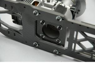
First tighten each of the four M3 bolts that attach the aluminum side engine mount blocks. When complete, remove them one at a time, apply blue Thread lock and then reinstall and tighten them.
