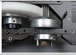
Install two #0061 bolts in the front and back open holes in the lower ratio plate and just snug them tight. Now install a #0060-1 6mm bolt in the remaining hole and just snug it tight.
