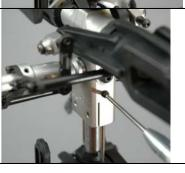
Finally, select the two #0067 M3 x 14 socket bolts, apply a small amount of blue thread lock and thread them into the clamp holes at the base of the rotor head. Tighten these bolts snug and then tighten an additional 1/8 turn to clamp the rotor head.
