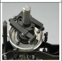
Take the fully assembled washout assembly and push it over the mainshaft on your model. Slide it down towards the swashplate. Take one of the link ends and snap it over one of the threaded balls on the inside ring of the swashplate. It doesn't matter which one at this point. Now repeat this procedure for the other washout link. This completes the assembly of the upper control system.
