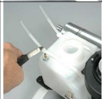
Grasp the fuel tank and align the mounting post with the grommet in the bottom frame plate. Square the tank to the bottom plate and seat it on the mounting tape.
