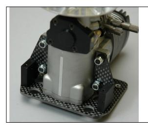
Select four #0080 M4 bolts and four #0021 M4 locknuts
