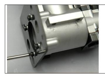
Apply a small amount of blue Thread lock to the exposed part of the bolts and attach the combined plates onto the engine back plate as shown.
