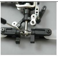
Hold the t/r hub and output shaft in this position and tighten the previously inserted dog point set screw on the other side of the t/r hub until it begins to engage in the t/r shaft.
