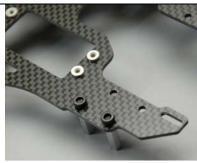
Insert the two bolts from the inside of the left frame through the two holes at the bottom of the gear drive cutout. Apply a small amount of blue Thread lock to the threads and thread the fan shroud spacers onto the bolts on the outside of the frame. Fully tighten using appropriate tools. These are the mounts for the fan shroud plate.
