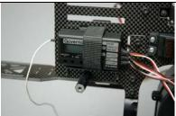
There is adequate room on the radio section of the frame to attach other accessories such as gyro amp, governor or regulator. Use double sided tape on the back of the device to stick to the frame and wrap it with Velcro tape routed through the frame openings to secure it.
