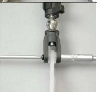
The t/r assembly turns at a very high speed and must be balanced before installation to ensure smooth operation. In order to balance the assembly, you will need a balancer of some sort like the one shown.
