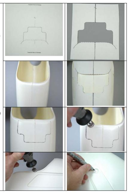
Using a marker, mark the center of each of the four canopy mount indentions in the canopy. You will need to drill a 17/64" hole on each of these four marks for the mounting grommets. It is suggested that you first drill a very small hole and then redrill the hole several times using progressively larger drills until you reach 17/64". You can also use a hole ream to open these holes. Using a knife or file to clean the edges of these holes so there are no sharp edges.
