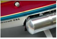
Hand fit the exhaust system to determine what if any cut-outs need to be made to the canopy. Mark the canopy and use a cutoff wheel or drum sander and a rotary tool to make any cutouts needed. Make sure there is at least 5mm clearance between any part of the canopy and the exhaust system.
