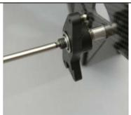
Using the #0061 M3 x 8 socket head bolt and #0003 M3 washer, apply a small amount of blue thread lock to the bolt threads and thread the bolt into the end of the bellcrank stud which will capture the bellcrank. Tighten the bolt firmly. Make sure the bellcrank moves freely. If it does not, check to make sure you completely seated the flanged bearings into the bellcrank.
