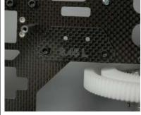
Select the left upper clutch plate and two #0060-1 M3 x 6mm socket head bolts. Position the plate on the left frame as shown and using a small amount of blue Thread lock on the threads, thread the bolts into the PEM mounting nuts in the frame half. Tighten both bolts firmly. Make sure you install the marked left plate on the correct side.
