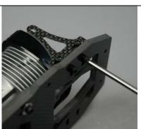
This step will install the fan shroud mount brackets onto the bottom plate assembly.
