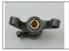
Now take the remaining clip and install it over the pitch slider. For best results, rotate it 45° from the first clip so that the retaining fingers don't align with the fingers on the first clip. This will ensure that this assembly does not come loose.
