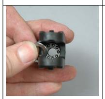
Select the ball cage from one of the thrust bearings and grease the inside of the cage (in the channel). Drop this bearing cage into the inside cavity of one of the blade grips so that this greased channel faces the thrust bearing race installed inside the blade grip.
