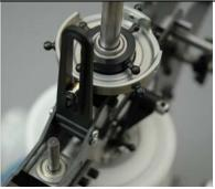
The swashplate should slide easily down the swashplate. Using a finger, slightly bend the plastic anti-rotation guide outward just enough to slip the bearing into it. When you release the guide, it will capture the anti-rotation bearing which prevents the outer swashplate from turning.
