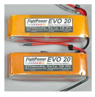
B) "C-rate". This is the rate at which the battery can be discharged. Most batteries currently available are good for at least a 10C continuous discharge rate, many are good for much more. Most setups in this helicopter will average 25 to 30 amp average current drains with bursts as high as 80 amps. Assuming a battery of 3700 mA and using the average of the first two numbers and the third number points to a needed continuous C rating of 7.4 and a burst rating of 21.6.
