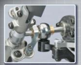
■ Every moving part of the tail rotor assembly is supported by precision ball bearings.
