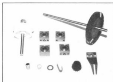
The ballraced bearing support blocks for the main shaft and gear.
