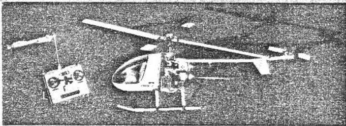
Completed Cricket and the Futaba radio that handled control inputs through S-20 servos; Super Tigre .25 engine for power.
