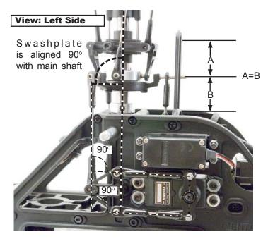
After installing the three cyclic pushrods, the swashplate should sit level.
