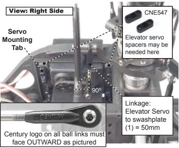
The elevator servo will mount with a half servo arm on the upper opening of the left side of the main frame. Use the 4 servo screws and 2 servo mounting tabs to mount the elevator servo with the servo arm output facing toward the rear inside of the frame (pictured above). The distance from the center of the servo to the center of the ball on the servo arm should be between 20-22mm
