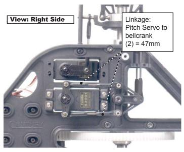
The aileron servo will mount with a full servo arm on the lower opening of the right side of the main frame. The distance between the steel balls (center of ball) on the servo arm should be 12.5mm. Use the 4 servo screws and 2 servo mounting tabs to mount the aileron servo with the servo arm further toward the rear of the frame (pictured above).
