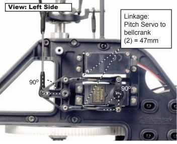
The pitch servo will mount with a full servo arm on the lower opening of the left side of the main frame. The distance between the steel balls (center of ball) on the servo arm should be 12.5mm. Use the 4 servo screws and 2 servo mounting tabs to mount the pitch servo with the servo arm further toward the rear of the frame (pictured above).
