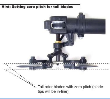
As the rudder stick is moved to the right, the rudder pushrod will move forward increasing the thrust in the tail blades rotating the nose to the right.
