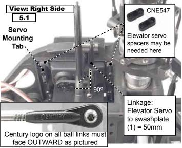
(5.1) The elevator servo will mount with a half servo arm on the upper opening of the left side of the main frame. Use the 4 servo screws and 2 servo mounting tabs to mount the elevator servo with the servo arm output facing toward the rear inside of the frame (pictured above).
