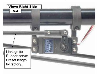
(5.4) The rudder servo will mount with a half servo arm on the servo bracket on the tail boom. Use the 4 Servo screws and 2 servo mounting tabs to mount the servo with the servo output facing the forward right side of the helicopter (pictured above).
