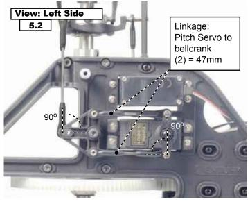
(5.2) The pitch servo will mount with a full servo arm on the lower opening of the left side of the main frame. Use the 4 servo screws and 2 servo mounting tabs to mount the pitch servo with the servo arm further toward the rear of the frame (pictured above).
