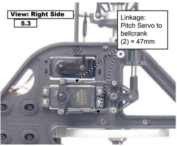
(5.3) The aileron servo will mount with a full servo arm on the lower opening of the right side of the main frame. Use the 4 servo screws and 2 servo mounting tabs to mount the aileron servo with the servo arm further toward the rear of the frame (pictured above).
