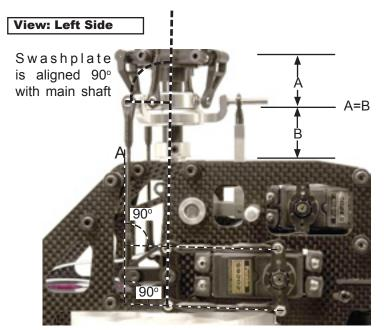
After installing the three cyclic pushrods, the swashplate should sit level.
