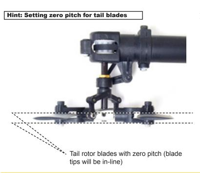
As the rudder stick is moved to the right, the rudder pushrod will move forward increasing the thrust in the tail blades rotating the nose to the right.
