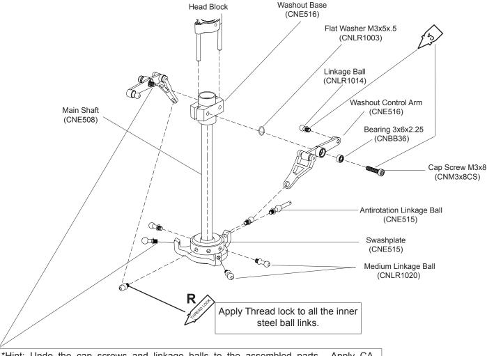
\*Hint: Undo the cap screws and linkage balls to the assembled parts. Apply CA on metal to plastic assembly. Apply blue thread lock on metal to metal assembly. Do not over tighten when screwing the attached assembly to its subassembly.
