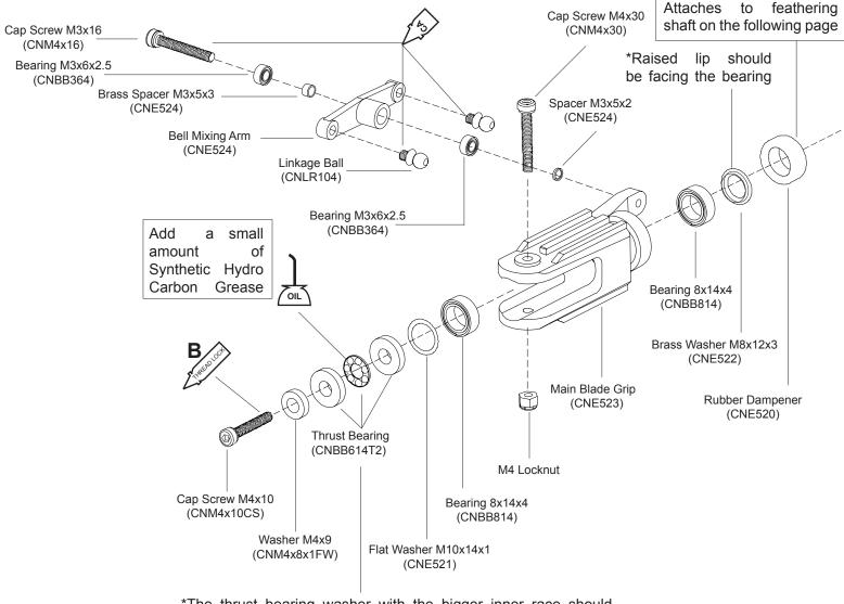
\*The thrust bearing washer with the bigger inner race should be closer to the head block. The thrust bearing washer with the smaller inner race should be closer to the rotor blade.
