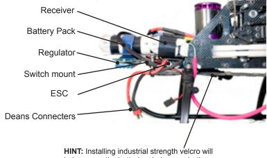
help secure the batteries during aerobatics.
