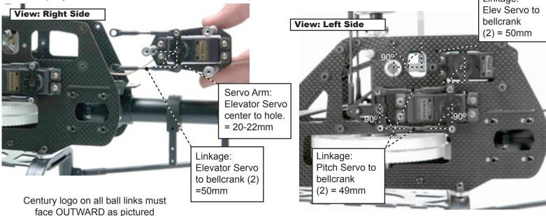
Use the 4 servo screws and 2 servo mounting tabs to mount the elevator servo with the servo arm output facing toward the front inside of the frame (pictured above). The distance from the center of the servo to the center of the ball on the servo arm should be between 20-22mm
