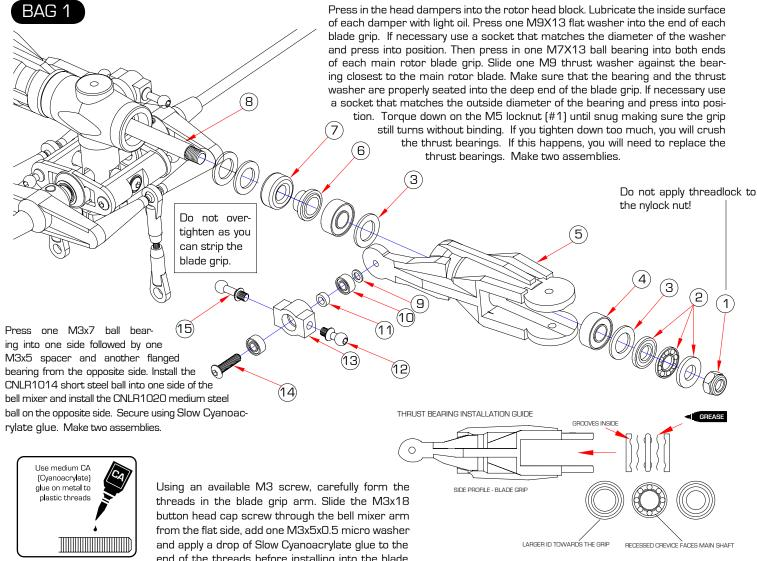
end of the threads before installing into the blade grip. Tighten the bolt until there is no end to end movement, but do not overtighten the bolt as you can strip out the hole. Make two assemblies.
