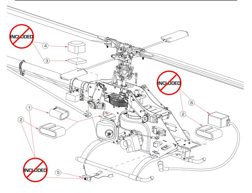
The electronics configuration is shown as an example of how to mount the electronics. It is not necessary to mount your electronics this way.
