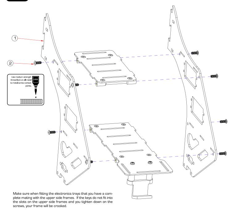
Apply medium threadlock to the eight M3x8 button head cap screws and tighten down.
