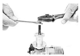
Tighten down on the top lock nut while applying opposite force (unscrewing) to the second nut using the Zenoah supplied wrench. This will allow you to lock the nuts together.
