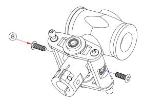
Do not secure all the screws until lining up the components in the following steps.
