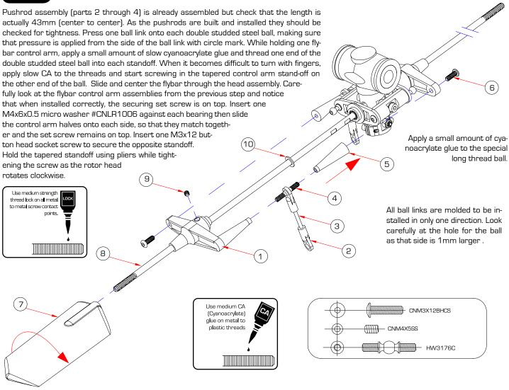
Loosely tighten the M4x5 set screws into the round aluminum inserts aligned with the flat spots on the flybar. Tighten both set screws, one at a time using Medium threadlock. Make a pencil mark 5mm past the threads on both ends of the flybar. Thread the flybar paddles onto the flybar until the mark is reached and align the paddles parallel. Again using the ruler, rotate one paddle or the other to get equal distances while remembering the leading edge of the paddles turn clockwise.
