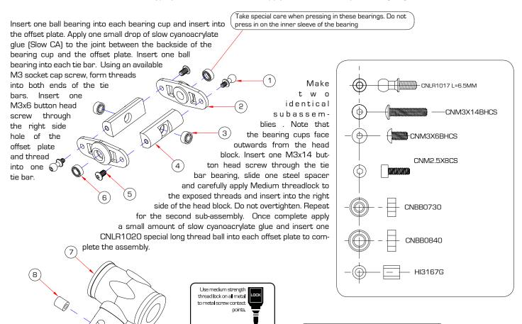
Do not secure all the screws until lining up the components in the following steps.
