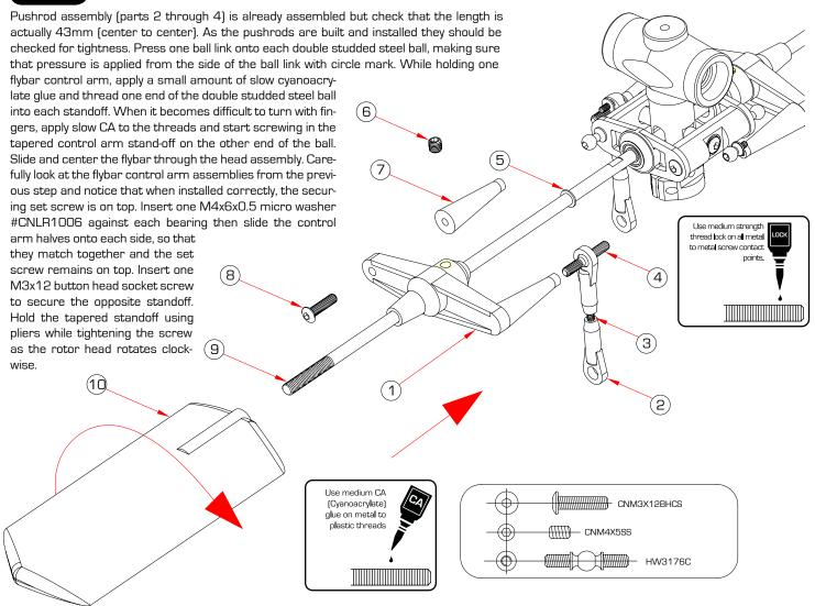
Loosely tighten the M4x5 set screws into the round aluminum inserts aligned with the flat spots on the flybar. Tighten both set screws, one at a time using Medium threadlock. Make a pencil mark 5mm past the threads on both ends of the flybar. Thread the flybar paddles onto the flybar until the mark is reached and align the paddles parallel. Again using the ruler, rotate one paddle or the other to get equal distances while remembering the leading edge of the paddles turn clockwise.
