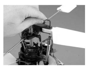
**STEP 3** Attach the Upper and Lower Rotor Blades using (1) M3x22 SHCS and (1) M3 Lock Nut per blade and 2.5MM Hex Key and 5.5MM Socket until snug and then loosen 1/2 turn. Blades should NOT be tight.
