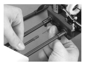
**STEP 8** Feed the Receiver Antenna Wire completely through the Antenna Protective Tubing (This step may require a firm piece of straight wire as a guide or pull).
