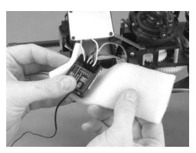
**STEP 5** Wrap the connected Receiver in the foam rubber as shown.
