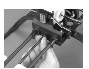
**STEP 9** Slide the flexible band on the Antenna Tubing until it just extends past the end of the tubing. Insert the tubing into the Tail Mount Panel. Check the antenna wire from Receiver to the Tubing for any obstructions.
