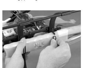
**STEP 15** Slide the connected Battery Pack forward into the nose of the fairing and secure with the remaining O-Ring Band. Note: The center of gravity of the AirScoot needs to be directly under the rotor shaft. Slide the battery around until the proper center of gravity is achieved.
