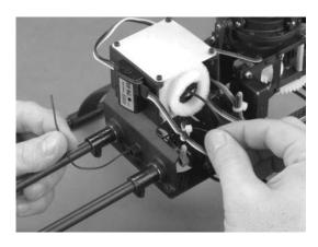
**STEP 7** Feed the Receiver Antenna Wire through the center hole of the Tail Mount Panel.
