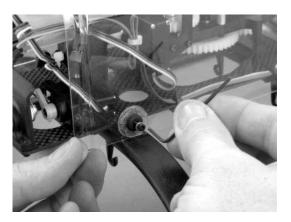
**STEP 12** Attach the Fairing to the Landing Gear Assembly using (4) Socket Head Cap Screws and M2 Washers as shown.
