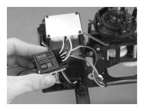
**STEP 4** Attach the Speed Control (#3), Rate Gyro (#4), Pitch (#2) and Roll (#1) Servos to the Receiver (not included) in the slot number indicated. See Appendix A to identify Control and Servo sources.
