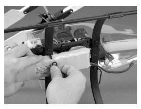
**STEP 13** Attach a charged 10-Cell 2400mAh Battery Pack (charger not included) to the bottom of the Base Plate using (1) O-Ring Band as shown.
