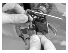
**STEP 14** Connect the Battery Pack to the Speed Control. DO NOT make this connection unless Transmitter is ON and immediate flight or checks (receiver channel connections, transmitter channel reverse, linkage adjustments, etc.) are planned. Always remove the blades when checking. Always disconnect immediately (with Transmitter ON) after flight or checks.
