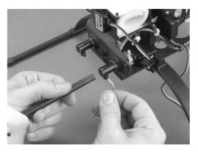
**STEP 2** Attach the Tail Fins to the Base Plate by inserting the Tail Fin Tubing into the existing socket (align fins vertically) and secure using a 2-5/16x1/2" SHCS and 2.0MM Hex Key. (Repeat process for remaining Tail Fin).
