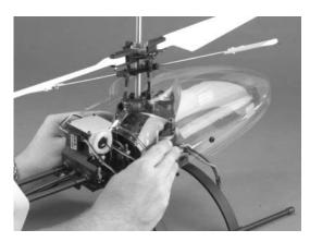
**STEP 11** Separate the rear portion of the Fairing Assembly and slide around the Main Rotor Assembly.
