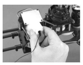
**STEP 6** Insert the wrapped Receiver into the upper compartment of the Tail Mount Panel with the Antenna Wire exposed as shown.
