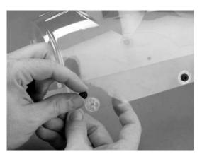
**STEP 10** (See Appendix B for fairing finishing instructions before installing washers). Using a hobby adhesive, attach (4) Plastic Washers to the inside of the fairing over the existing holes. Once secure, insert (4) Rubber Grommets.
