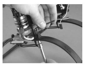
**STEP 1** Attach the Base Plate to the Landing Gear Assembly using (4) M3x16 SHCS and (4) M3 Lock Nuts, 2.5MM Hex Key and 5.5MM Socket as shown.
