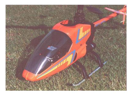
The 'Maverick' first appeared at the 1990 Sandown show in un-named and incomplete, .60 powered, experimental form and drew some favourable comment. A feature of the model was the use of a mechanical CCPM system in which all three of the pitch servos rose and fell with the swashplate. At that time, Jim Morley's company was going through some extensive reorganisation which meant that there was no finance available to develop the model further.
