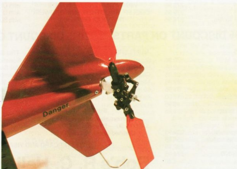
Tail rotor unit. A very nice working unit too. You will also note it is on the retracting blade side for a A.C.W rotating model. Shigetada Taya's model made use of this principle also but on the opposite side. Photos by: Lance Lewis.
