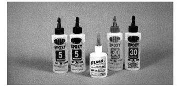
You will need two types of adhesives for the civil MD530 Epoxy and Instant (cyanoacrylate) adhesives. We recommend that you purchase both 5-minute and 30minute epoxy to cut down on assembly time, but you can get by with only 30-minute epoxy if time is not important. You will also need a small bottle of both "Thick" and "Thin" instant CA adhesive.
