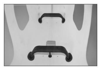
4. Remove the landing skid assembly from Heli. Remove the brace from the aluminum strut. Do not remove the strut and skid pipe as they are already adjusted and secured. Place the brace in place and install the strut and skid pipe onto the brace. You may apply Vaseline on Silicon Fairing to increase the lubrication for easier installation.
