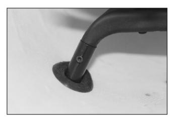
5. Secure the Aluminum Strut and Brace with 2.6x14mm Socket Screw. Hint: Install the left Aluminum Strut Assembly and Brace first. Pull the brace out and secure the socket screws then push it back and pull the right side out then install the right aluminum strut assembly.
