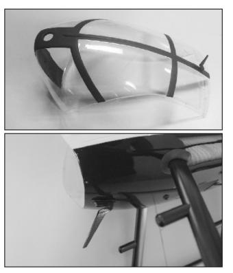
19. Install the wire strike on the front windshield. The big one is at the bottom and small one is on the top. Use 2x5mm wood screws to secure the strike in place.
