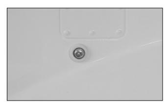
15. Secure the fuselage with 3x10mm washer selftapping screw as shown.
