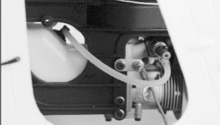
18. You will have to install the remote glow plug adaptor (TTR3803) for easy glow ignition. Also install a diverter and drill an exit hole at the bottom of the fuselage or you may extend the diverter to fuselage exhaust ventto obtain a more scale-like look.
