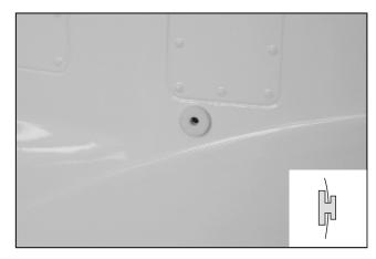
11. Drill the hole on the molded dot. Next enlarge the hole at about 8mm in diameter. Insert the Silicon Grommet on the hole. The smaller side faces outside.
