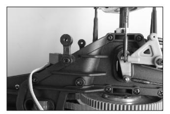
10. Remove the tail rotor assembly and proceed to extract the Raptor from fuselage. Replace the old post with the new plastic post mount with 3x18mm self-tapping screw. Place the Raptor into the fuselage again, the post should be located near a molded dot on fuselage.
