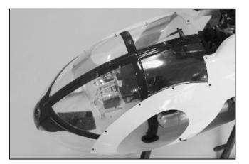
20. Install the front windshield with twenty 2x5mm screws and M2 nuts. Carefully make drill marks and drill 5/64" (2mm) holes then secure the front windshield in place. Apply thin instant CA adhesive for each screw and nut.
