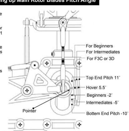
The total pitch angle range should be at  $-10^{\circ} \sim +11^{\circ}$ .
