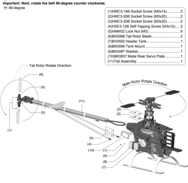
Pull the belt through the tail base, keeping the belt correctly aligned. Push the tail boom into the tail base all the way to the end. Place the drive belt over the tail drive spur gear. Then, gently pull back on the tail boom until the tension on the belt allows no more than 5mm(3/16") of free play in the belt. Tighten the locknuts and proceed with the rest of the assembly.
