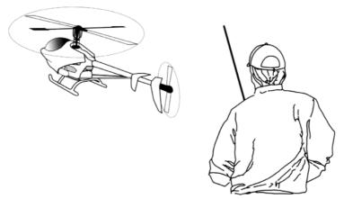
(2) Always stand behind the model helicopter when learning how to hover. Then you can watch the nose of the helicopter. A left tail rotor command will yaw the helicopter nose to the left, and a right command will yaw to the right. Similarly, a left cyclic command will cause the helicopter to translate left. After you can comfortably hover the model at one meter high without drifting, then start practice hovering while standing to either side of the model.
