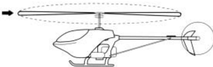
(3) When both blades are in track, the blade tips will appear to overlap as seen from the edge of the rotor plane.
