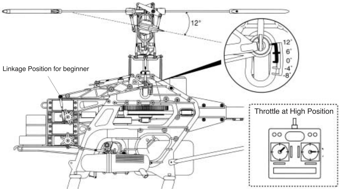
Move the throttle/collective stick to the full throttle position(see upper right diagram). The molded "pointer" should now line up with the upper limit mark, which should provide about 12° of blade pitch.
