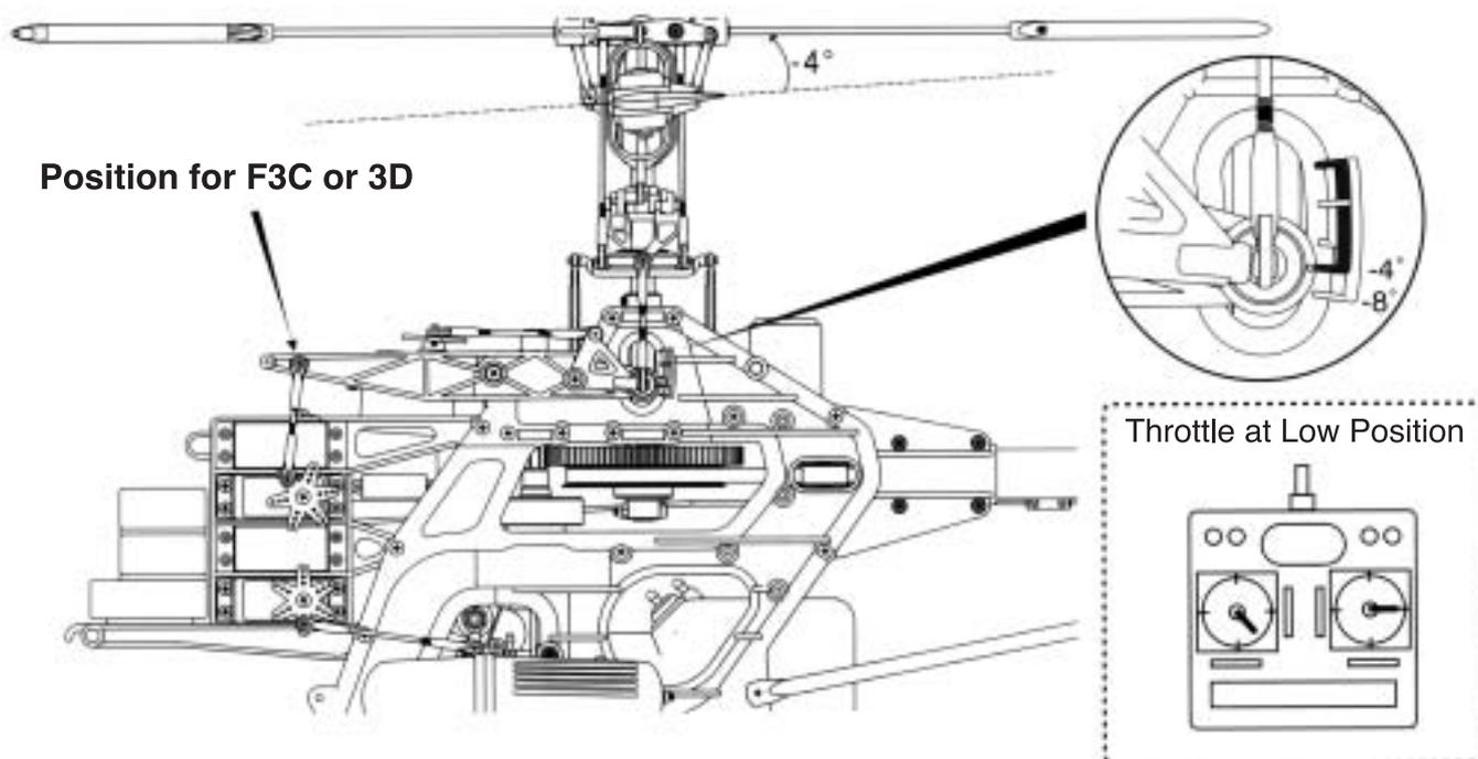
For intermediates set the low end to  $-4^\circ$ . For advanced F3C and 3D flying, set the low end to  $-8^\circ$ .
