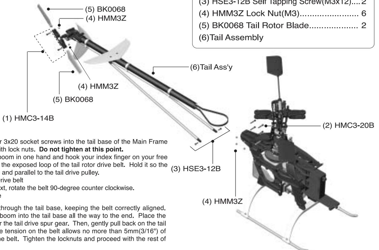
Insert the four 3x20 socket screws into the tail base of the Main Frame and secure with lock nuts. **Do not tighten at this point.**
