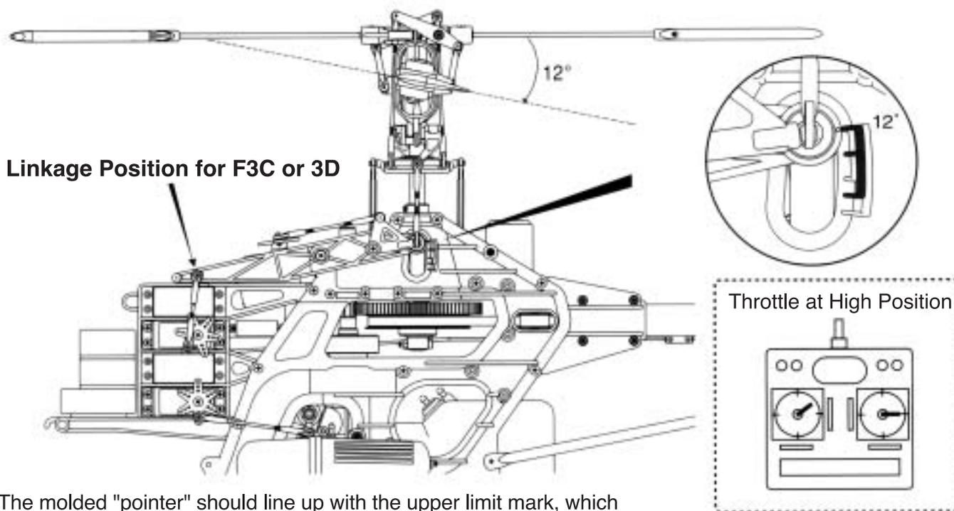
The molded "pointer" should line up with the upper limit mark, which should provide about  $12^\circ$  of blade pitch.
