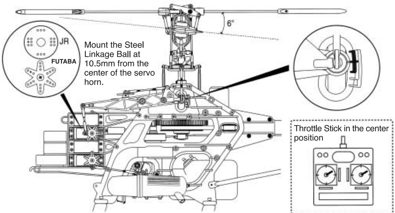
6° hovering pitch angle is used for beginners, intermediates and experts. The throttle/collective must be in the center position when adjusting the collective pushrod length to make the "point" line up with the 6° hover point on the molded scale (see above diagrams).
