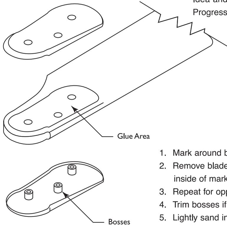
1. Mark around blade grips with a felt-tip marker.
