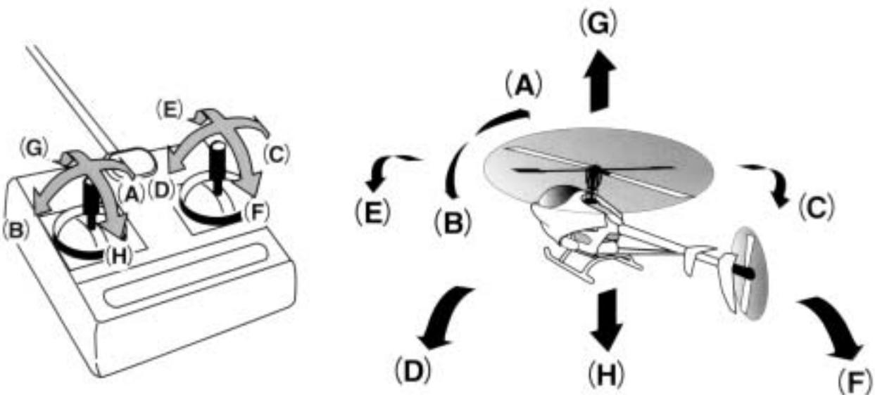
Always check all the controls to make sure they move in the correct direction and there is no mechanical binding or noise from the servos.
