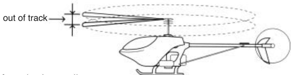
If the blades are out of track, then adjust one of the pushrods that connects to the main rotor blade pitch arm.
