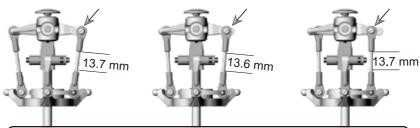
Different ball head installation on grip lever affects flight response, adjust position according to personal preference.
