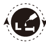
General thread lock. Tighten screw and apply thread lock. 一般型止鬆劑
