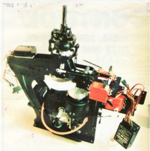
Another view of the mechanical assembly. This unit drops into the fuselage, is mated with the tail drive and then bolted to wooden bearers. A fairly simple task.
