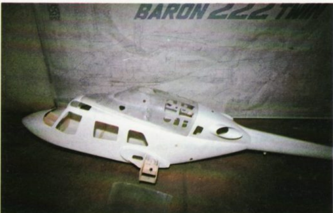
Main body after first coat of primer. Although some pinholes showed up in the gel coat of the fuselage, these were easily filled with powder and paint mix.
