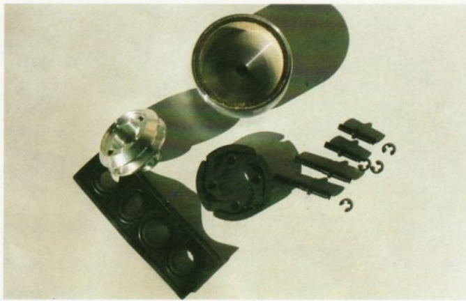
Clutch bell and shoes. Note the super thick clutch bell lining. The rubber strip gives four O rings which give different degrees of clutch pick up to the main gear drive.
