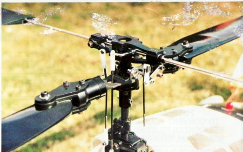
The K3SB Black Head with 2mm plate. Twin ballraced blade holders and ballraced flybar ensure positive response.
