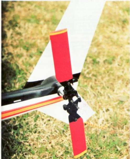
Tail unit /blades. This is totally slop free, and very smooth in operation.
