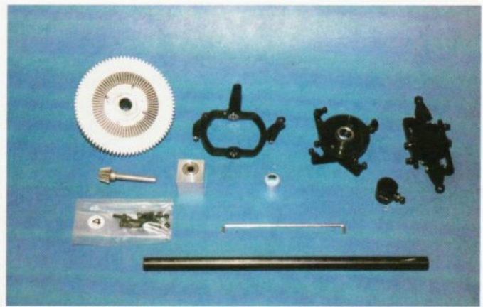
Main gear with steel tail gear insert. You won't strip this unless you plow in to the ground head first from a great height. Swashplate, mixer unit, and shaft are all high torsion steel and superbly crafted.
