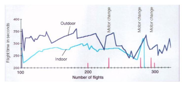
Fig.1 Comparison of indoor and outdoor flying times on 1100 mAh battery.
