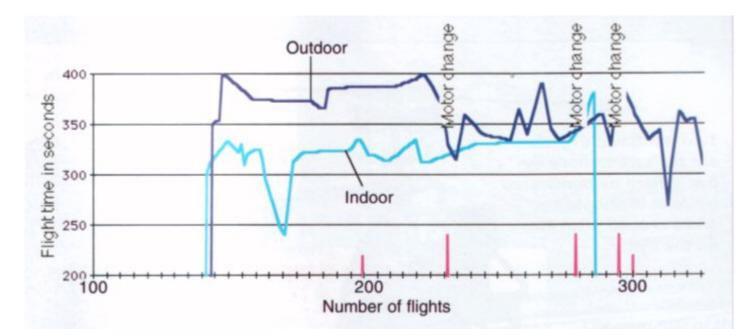
Fig.2 Comparison of indoor and outdoor flying times on 1400 mAh battery.
