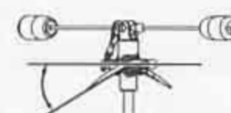
If it turn counterclockwise, increased pitch angle
