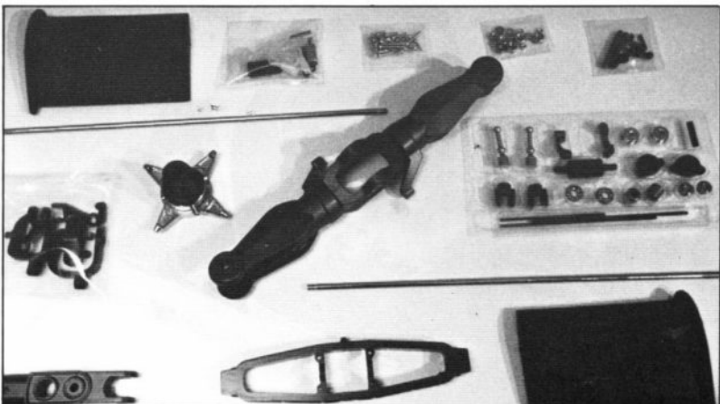
The rotor head components laid out prior to assembly, tail blade holders, swashplate and scissors link.
