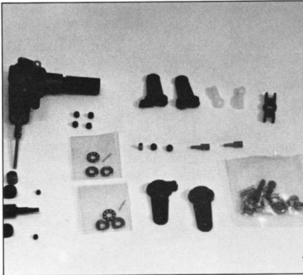
Tail rotor gearbox with blade holders with double ballraces.
