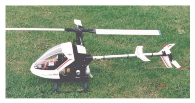
The original Robbe/Schluter 'Moskito' kit was supplied wit both skids and a tricycle undercarriage, together with a plastic cabin/canopy unit with an integral dummy pilot. A notable feature was the possibility of building the machine for clockwise or anti-clockwise main rotor direction. This kit is still available as the 'Moskito Standard'.
