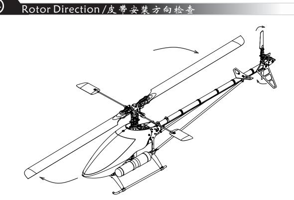
When Main Blades turn clockwise, tail blades should turn clockwise when view from the Tail Fin side. If not the belt is installed incorrectly.
