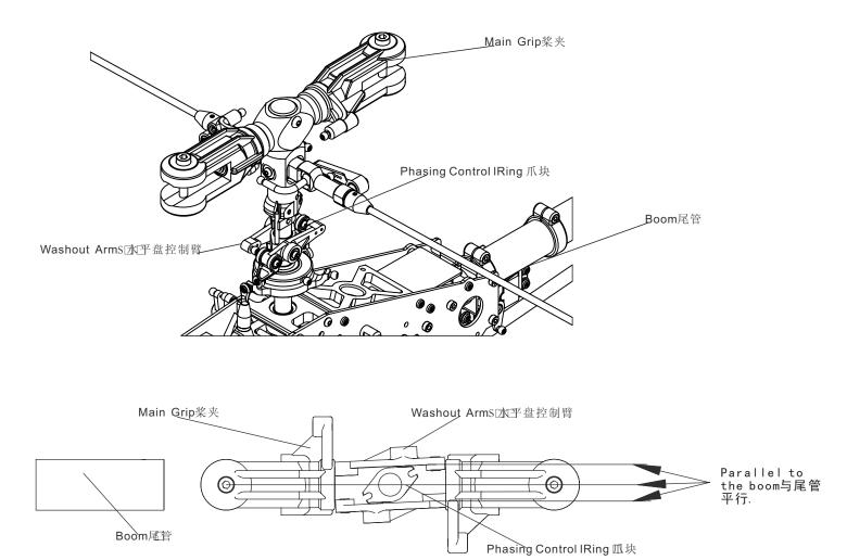
爪块控制组设置的角度应保证水平盘控制臂与桨夹同时平行于尾管. Get the right phasing adjustment by turning the phasing control ring until the Washout Arms and Main Grips both parallel to the Boom.
