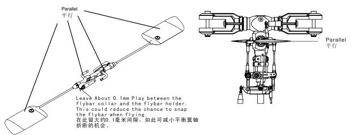
**Make sure the flybar control arm and paddle are in line as in the diagram.** 保证平衡翼控制臂和平衡翼相互平行,开始设定.
