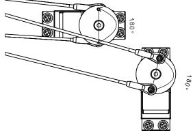
Note: The 2 Push-pull link rods are not necessarily parallel, but must be the same length. 注意:双推拉连杆不一定要平行,但长度一定要一致.
