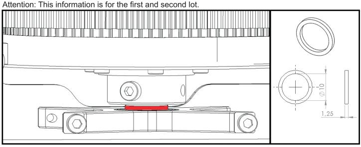
This 1.25mm thick spacer-ring need to be assembled between the oneway-sleeve and the lowestet bearingblock.
