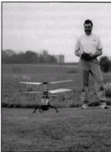
*Harris Malkin hovers AirScoot after adjusting rotor ball links, and setting and initializing gyro.*
