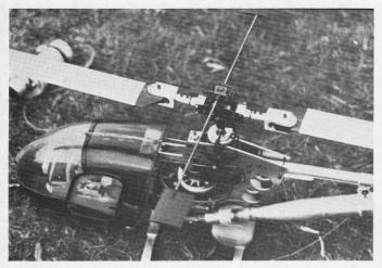
model helicopters, possibly the most relevant virtue of a lead lag hinge is that it may save you a broken blade when your model topples over, so why aren't they fitted to all blades? Well, there is a great deal to be said for having your blade in the right place from the point of view of control response and load feedback into your swashplate linkage servo system and the forces described can vary by about 16 times from one design of model to another, making it almost essential on some set-ups.
