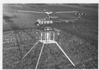
Above left: the Dave Nieman lead/lag rotor blade hinge mentioned in text 'New Trend,' fitted to a DS222. Above: this West German training aid, the Helfe Mechanick, has a telescopic pillar and is free to rotate. Adjustable stops and spring restraint allows gradual progress to greater freedom.
