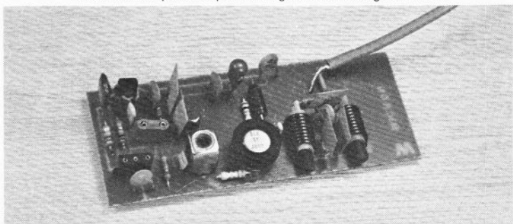
The completed R.F. section is shown above, while below may be seen the whole “works” of transmitter—less nicads and case.
